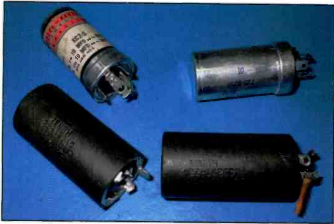
Photo B. The two FP capacitors removed for rebuilding. Two NOS caps, shown below, will be gutted and used for the restoration. They are new, but still are at the end of their life-cycle after decades of storage. I save them for rebuilding instead of tossing them out.
