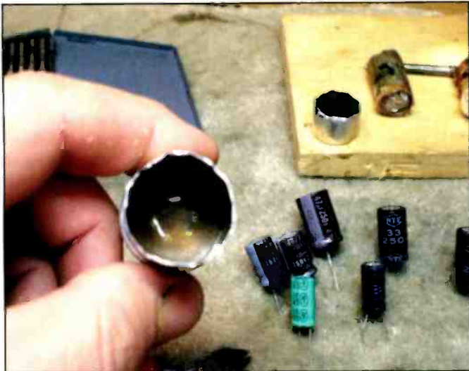
Photo E. I cut the metal cans open using a sharp utility knife. Once exposed, the old electrolytic capacitors were removed and discarded. The old capacitor body can be seen on the wood board at the rear of the photo.
