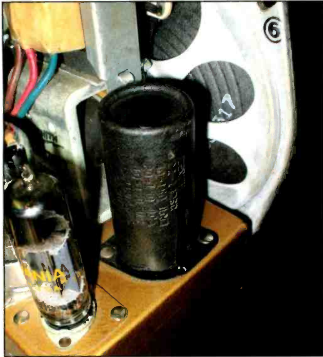
Photo H. Space is tight and all of the available room was needed to house the three replacement caps in this can. Note that heatshrink tubing or insulating "spaghetti" covers any exposed leads. A few dabs of hot glue hold the parts in place.
