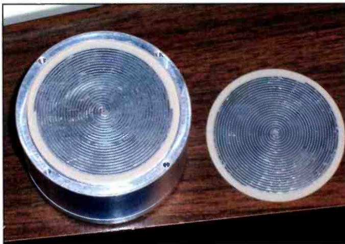
Photo A. Spiral antennas for a missile decoy.
