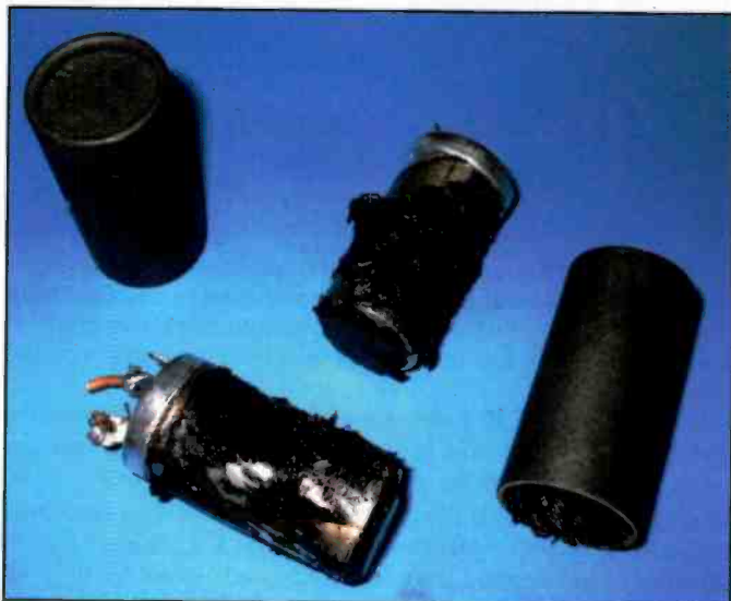
Photo D. The cardboard capacitor insulators after removal. These will be reused, so be sure to put them aside and save them.
