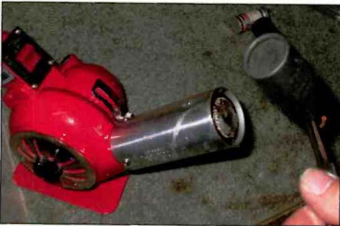
Photo C. Gently heating the cardboard tube while constantly rotating the capacitor body assures even heating. Once the tar is softened the cardboard shell easily slides free of the metal can.
