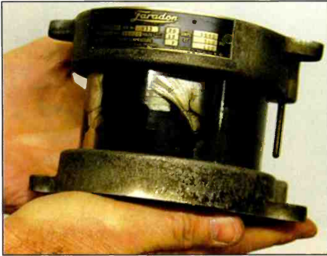
Circa 1939 Faradon capacitor once used for phasing of a directional antenna array.
