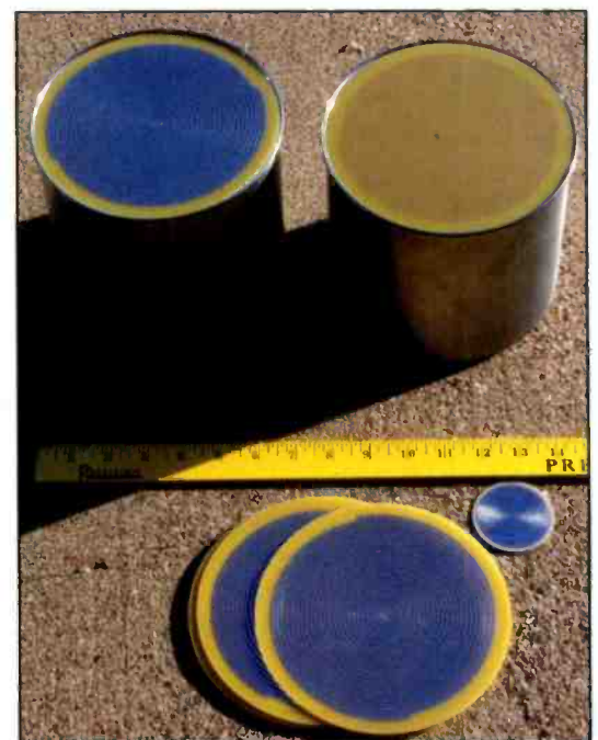
Photo B. Spiral antennas for an antenna test range.
