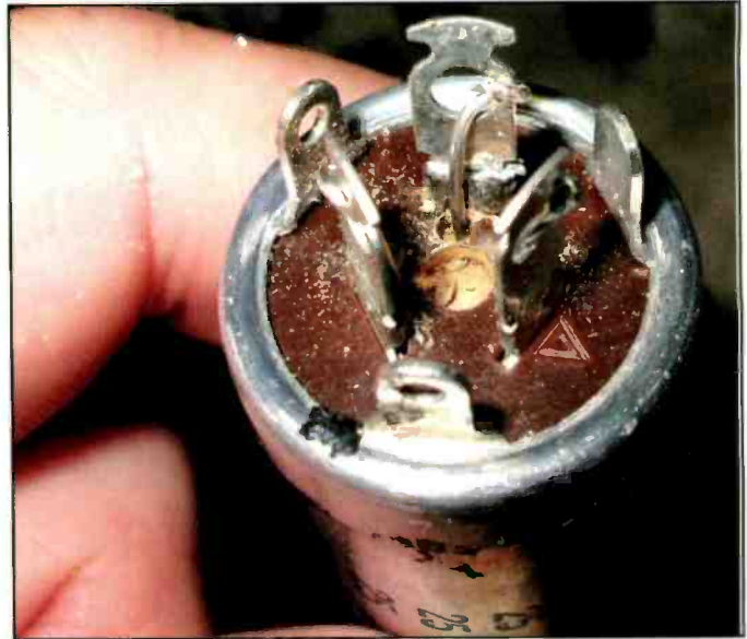
Photo G. If you looking closely you can see how the wire leads from the new caps pass through the holes and wrap on the adjacent solder lugs.
