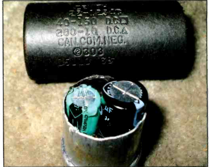
Photo I. Once the original cardboard shell is reattached it becomes almost impossible to tell that the part was ever disturbed! Yet, the cardboard can be quickly removed if the capacitors ever need to be replaced in the future.
