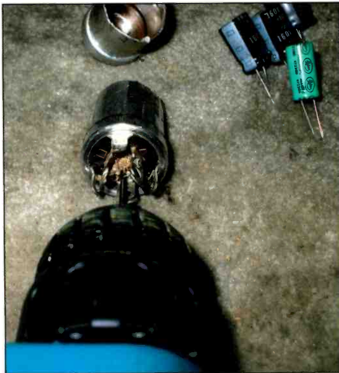
Photo F. Because the replacement caps will be hidden inside, I use a drill to make small wire gauge holes for the new leads to pass through. These will be soldered to the lugs on the base insulator.
