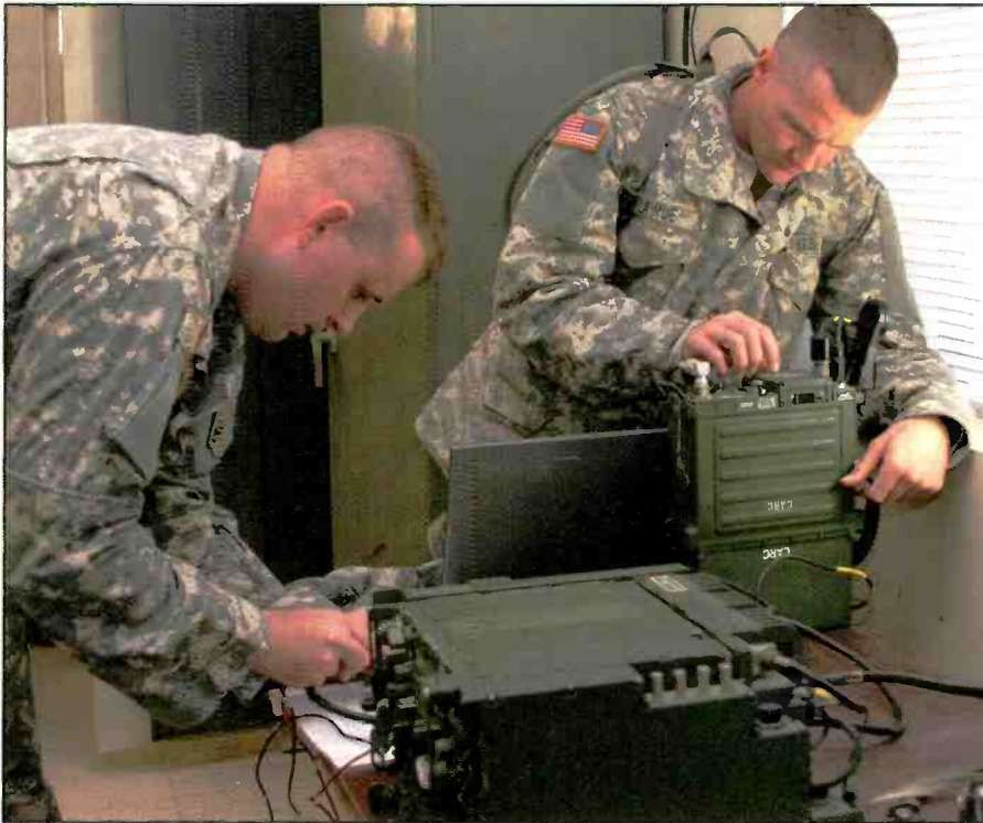
Instructor (left) and a student troubleshooting SINCGARS radios in a Tactical Operations Center.
