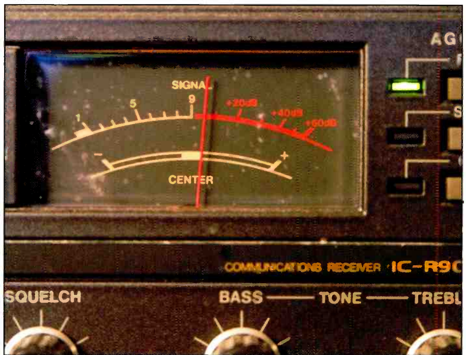
A good old-fashioned S meter comes in handy when you're experimenting with antennas, because it can help to confirm what your ears are telling you. Don't worry if you don't have one, though—just listen carefully and take your time.
