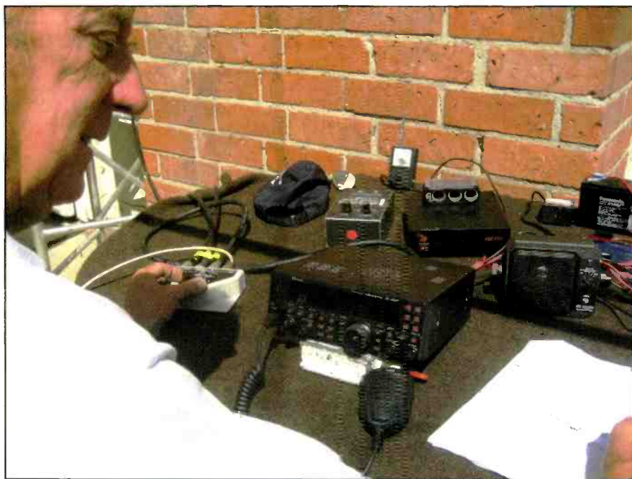
Gordo testing the Yaesu FT-450 during a ham class in the back yard. It put out over 130 watts on a whistle.
