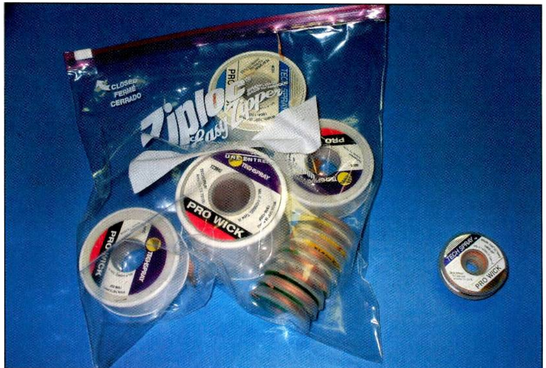
Photo A. Store unsealed solder wick spools in airtight sandwich or freezer bags to reduce oxidation on the copper braid. This will keep the wick working as good as new. Empty spools will hold several feet of solder for use with portable gas soldering irons.
