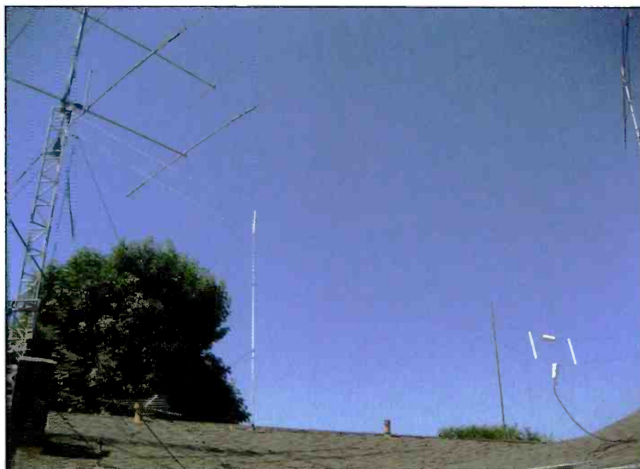
Gordo compared the B & W folded dipole (white spreaders) to a simple homebrew dipole. The dipole won on transmit, but the B & W did a lot better on receive.
