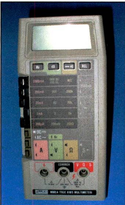
Photo C. By the 1980s, True RMS meters were becoming practical and affordable. It's hard to believe, but I've owned this meter since they were first introduced! While it can handle complex AC waveforms, it will not accurately calculate the RMS voltage if a DC component is present.
