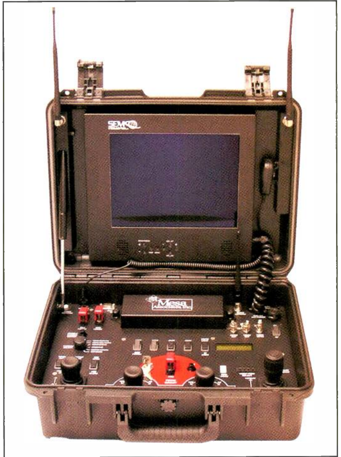
The briefcase operator control unit for Mesa Robotics' Matilda II. Note the video display screen and multiple joysticks, as well as the wide array of switches and indicators that allow complete control of the robot. More recent versions use the 900-MHz band for control, and 1.8 or 2.4 GHz for the video feeds. (Photo courtesy Mesa Robotics)
