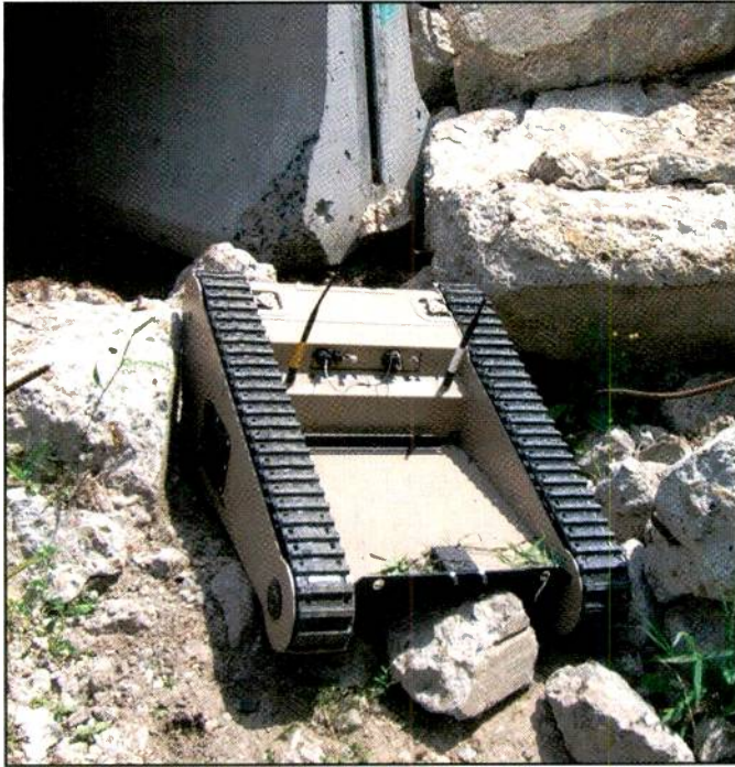
Mesa Robotics' Matilda II Search and Rescue Robot is shown maneuvering through extreme rubble during the DHS/NIST-sponsored Response Robot Evaluation Exercise at Texas A&M's "Disaster City" training facility. (Photo courtesy Mesa Robotics)
