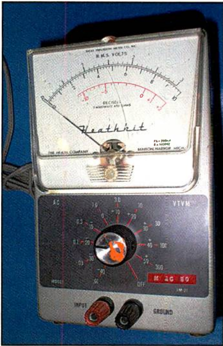
Photo B. Heathkit's model IM-21 AC vacuum tube voltmeter was designed for measuring very low-level AC voltage and has a greater frequency range than most general purpose VTVMs.
