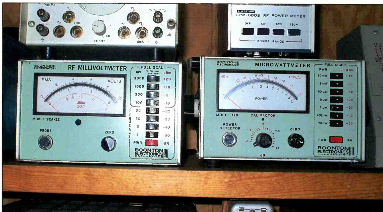
Photo E. These two Boonton meters were designed for low-level RF voltage and power measurements. Once again, they're extremely common on the surplus market and sell for very modest prices.
