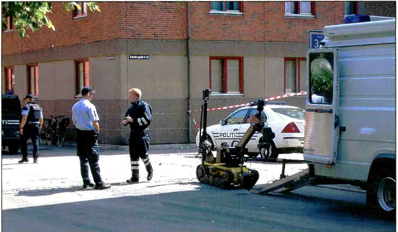
A Danish bomb robot, known as a rullemarie, enters a transport vehicle after completing its mission. The robot is remote-controlled from the vehicle and can be equipped with different kind of tools depending on the situation. (Photo via Wiki Commons)
