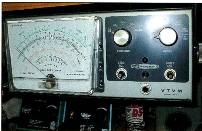
Photo A. My Heathkit IM-13 vacuum tube voltmeter has served me well since I built it from a kit in the 1960s while I was still in junior high school!
