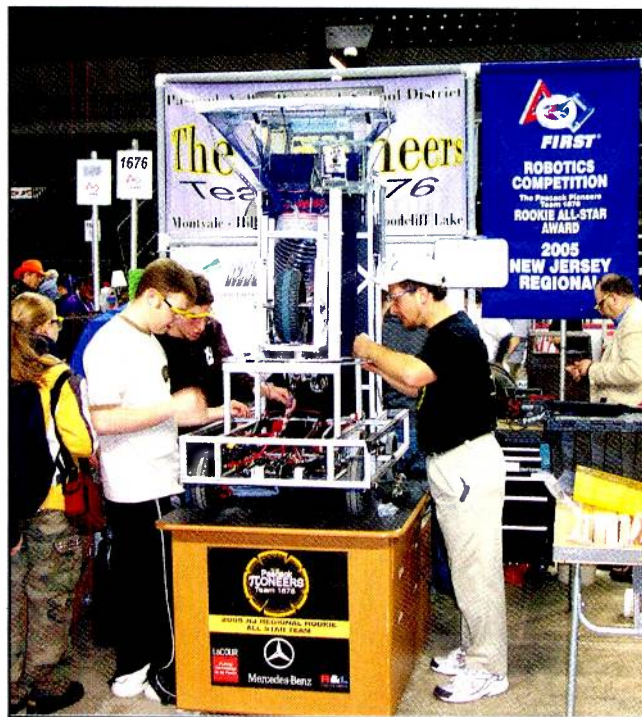
Students and a mentor work on their robot at the 2006 FIRST New Jersey regional competition. This robot was designed to collect and shoot 8-inch foam basketballs at a target 10 feet in the air.
