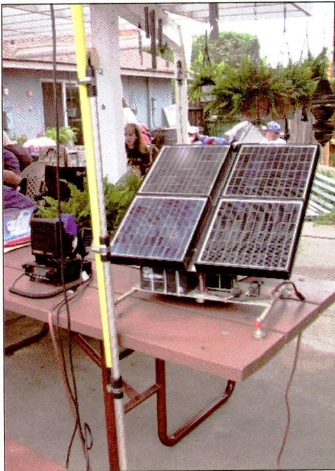
This sun-seeking solar array is good for 2 amps.
