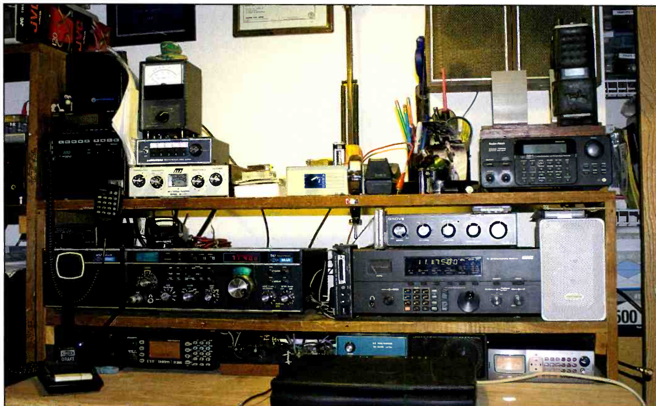
...but elaborate isn't necessarily a bad thing. This is the author's home station, with a Drake TR-7 monitoring the 40-meter ham band, and a Drake R-8 receiver tuned to 11175 USB. A variety of other useful radios is also visible.
