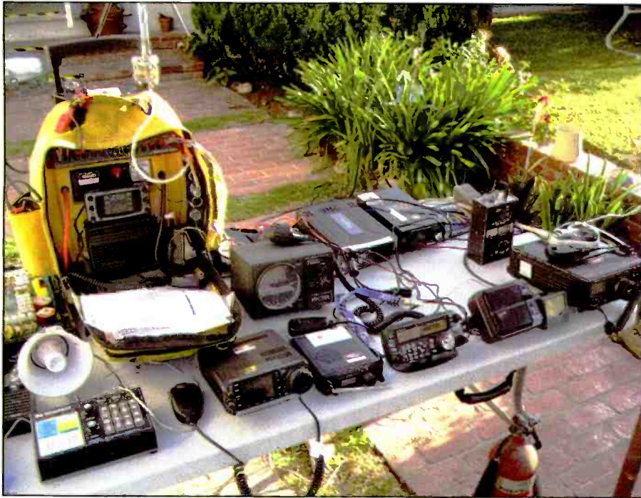
For a recent outdoor event, this classroom demo gear ran all weekend on solar and gel cell battery power.
