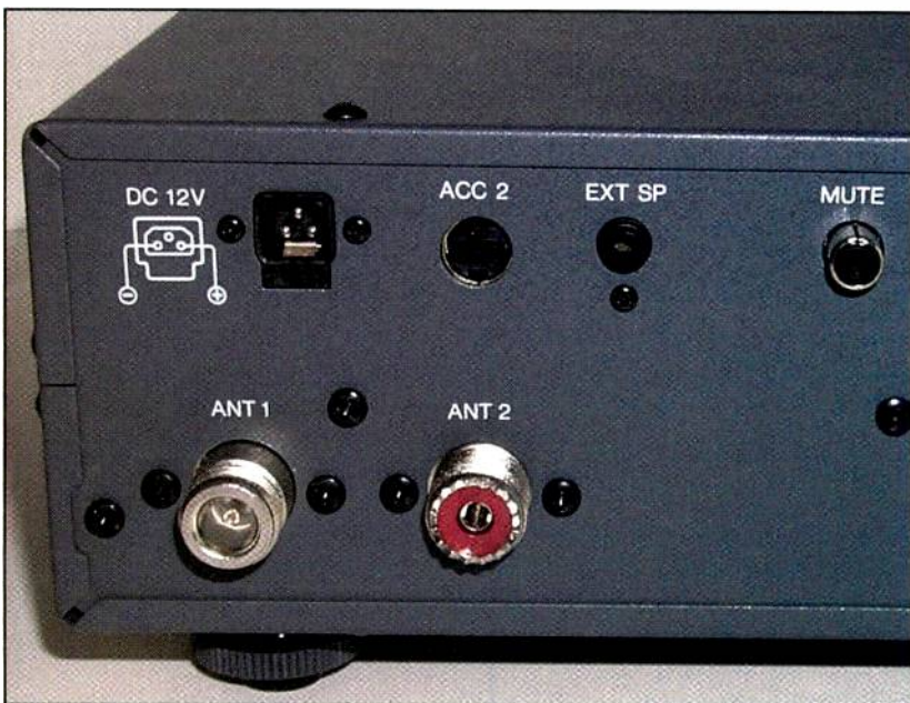
Most base and mobile scanners made in the last several years, including this AR-5000 base unit, can be powered by DC from the car. Note, however, that this one requires a special cable; most do not.
