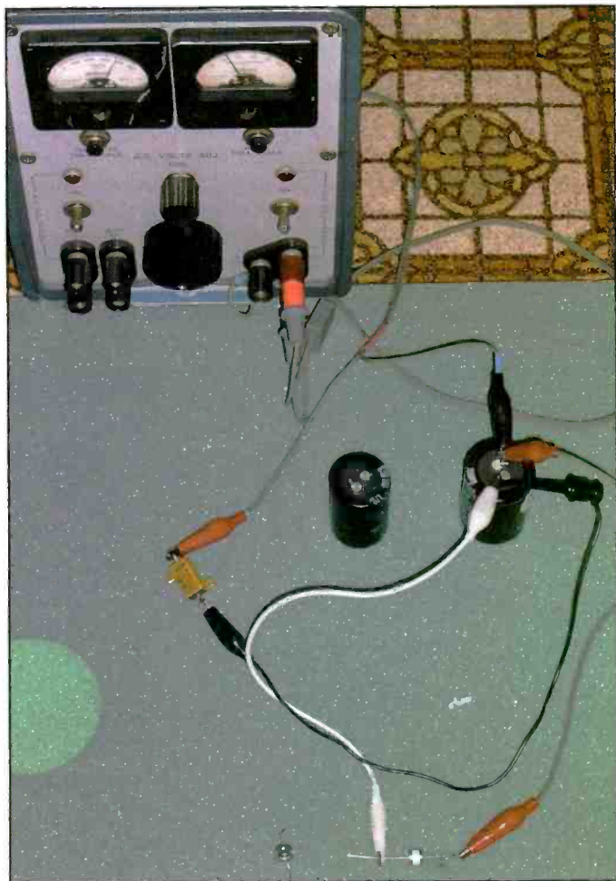
Photo D. My gas discharge tube stress tester.
