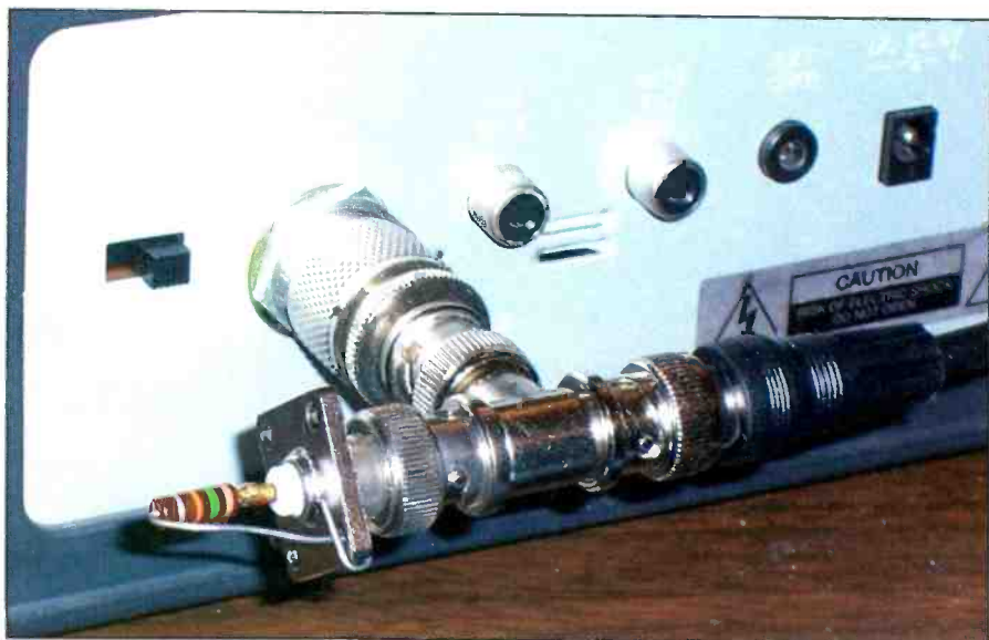
Photo F. Simple static dissipater for SWL radios and scanners.
