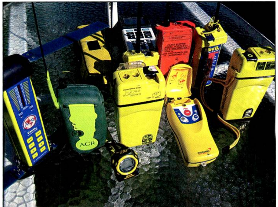
All these 406 MHz emergency locator beacons also transmit on 121.5 MHz.
