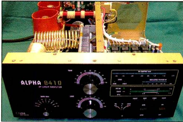
Alpha Radio Products new AP8410 is a 1.5 kW tetrode HF amplifier.
