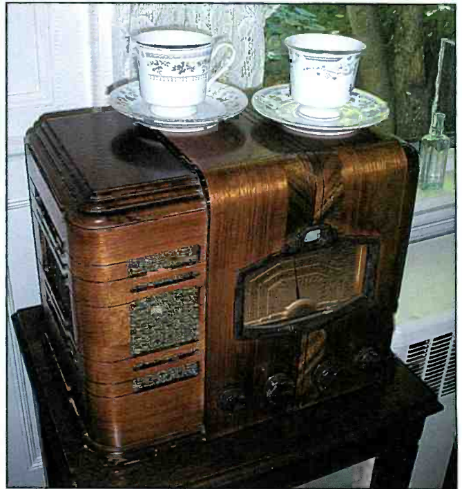
Photo I. Silvertone model 7463 from the mid-to-late 1930s, featuring both AM broadcast and shortwave bands and a "tuning eye."
