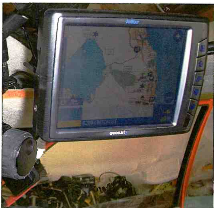
One of the two GPS units in the mix, this one featuring an AvMap display and located in the visor space overhead.
