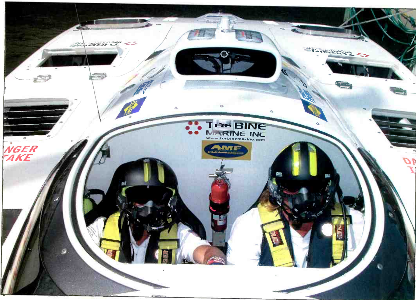
High-speed boat racing is not for the faint of heart. The crew of Miss Geico, a race boat with two 1800 HP turbines that gives it a top speed of around 190 mph, wear face masks with integrated breathing and communications devices. (Photo courtesy of Ron Polli)
