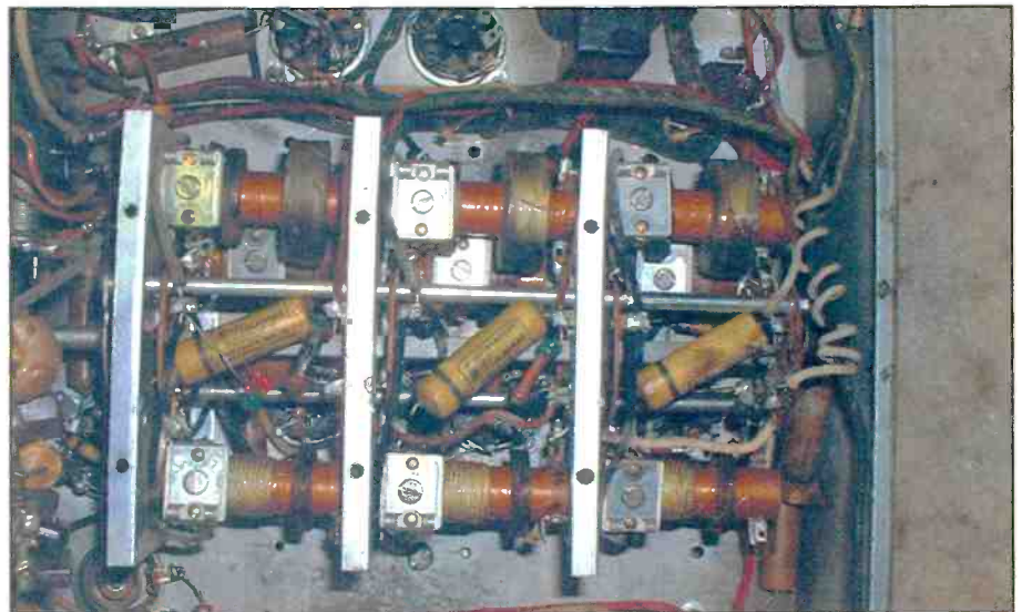
Photo D. Here's a view of the full IF-RF voltmeter channel band-switch assembly. Sharp eyed readers might note that in addition to the damage illustrated in Photo C, the plate dropping resistor at the other end of the assembly also shows severe signs of overheating—another failing wax cap at play. The entire assembly needs to be removed to reach hidden bypass capacitors on the tube sockets below; Photo E shows more detail. Several wax caps in the switch assembly also had to be replaced.
