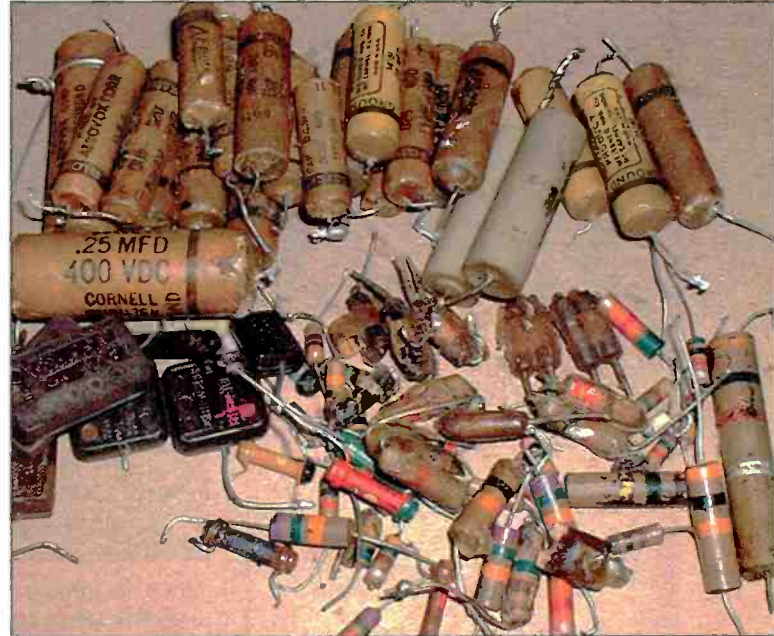
Photo C. This is the pile of resistors and capacitors that were replaced during the restoration. There was much more involved than I had envisioned.
