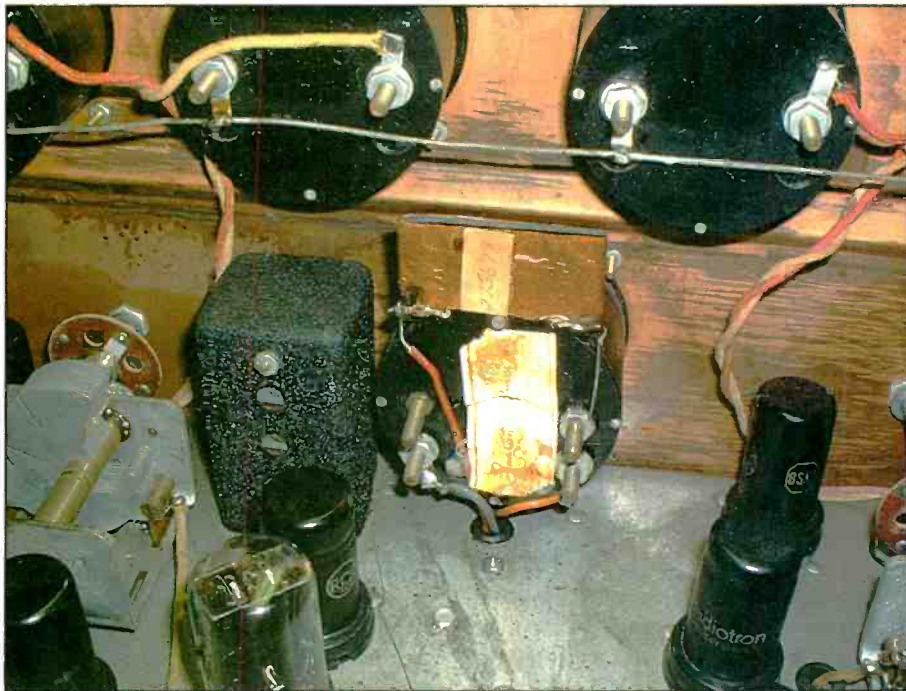
Photo G. A behind-the-panel peek shows that the external precision wire-wound resistor that's in series with the AC supply voltage going to the moveable coil in the meter movement. The meter bears a serial number, giving some indication that these were relatively expensive wattmeters. Hickok only used them in early Traceometer models.
