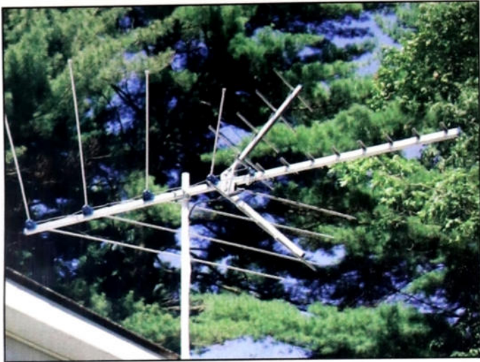
A familiar but old-fashioned Yagi-style VHF/UHF outdoor TV antenna wasn't up to the task of DTV reception.
