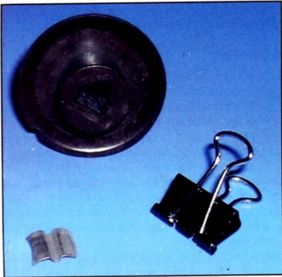
Photo B. The spring steel used in this style paper clip is an ideal source of tempered spring steel to make knob shim replacements. The material can be cut to fit using aviation tin snips, and shaped with needle nose pliers. A slight curve is needed.
