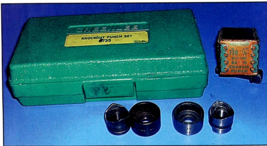
Photo C. In this photo a Greenlee 7/8-inch radio punch (right) is compared to an electrician's 1-1/2-inch knockout punch. Notice that both punches are identical! Radio punches are marked by the size of the hole they produce, while electricians' punches are marked by conduit size! Beware the difference.
