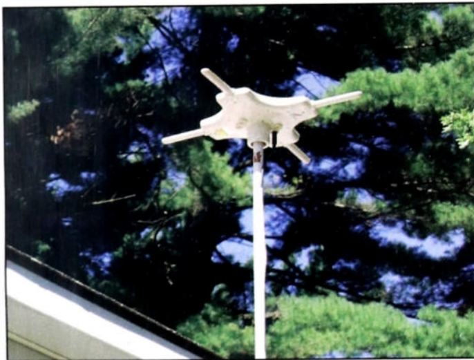
I replaced the old Yagi with a modern-looking DTA-5000 UHF/VHF Smart Antenna for significantly improved DTV reception.
