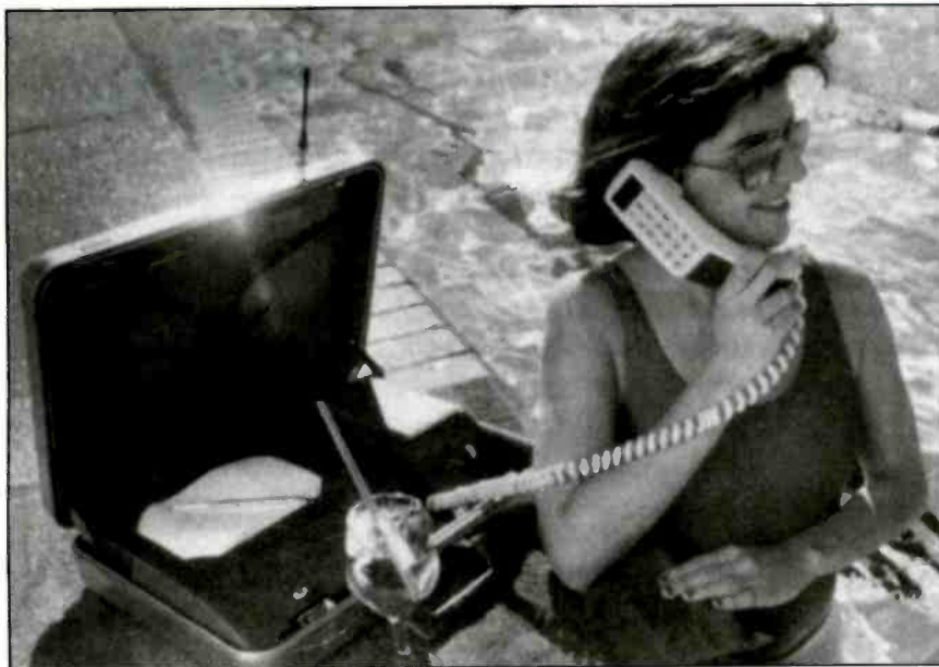
Photo B. A briefcase analog cellular phone circa 1985. Thirty pounds of pure communications sexiness—if you could afford the $3,000 price tag. This beauty was an early NEC cellular car phone stuffed into a metal briefcase with over 10 pounds of lead-acid batteries and a charge controller.
