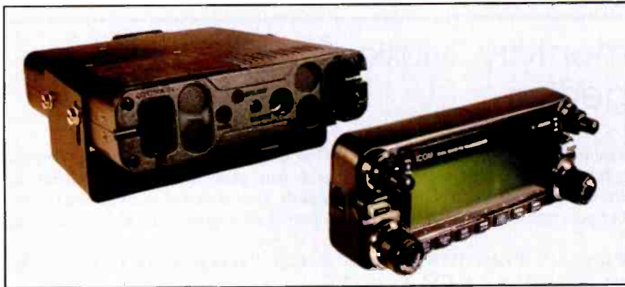
The removable control unit makes this a great rig for mobile use.
