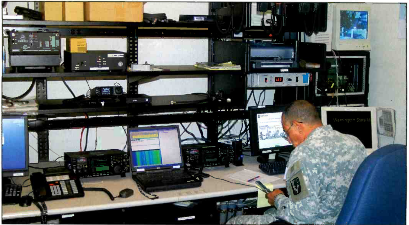
SSG Delgado-Rosario monitoring the HF radio system while preparing to contact the armories throughout Washington State. The Harris radio is located on the far right with the ICOM radios in the center. The computer is used for MT-63 digital communications during our MARS net.
