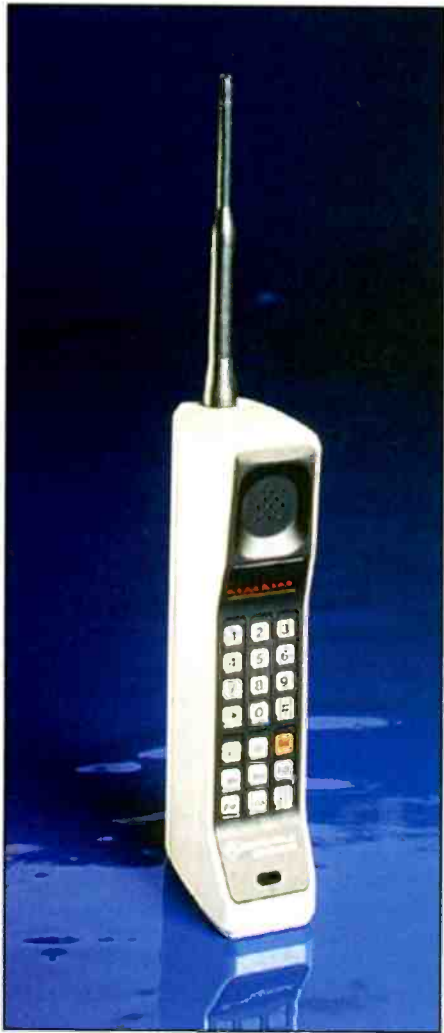
Photo C. This Motorola DynaTAC 8000X was the first handheld AMPS cellular phone to win FCC type-acceptance. It cost $4,000 in 1984 and its maximum RF power output was limited to 600 mW because of health concerns about microwave energy on the brain. Vehicular and transportable cell phones had a full 3-watt maximum RF output.
