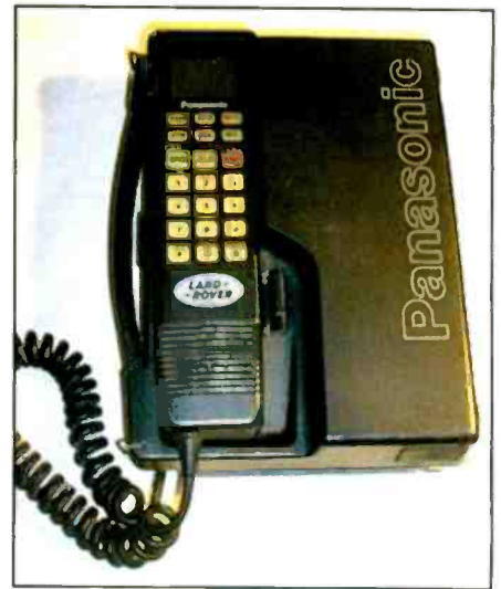
Photo D. A Panasonic transportable AMPS cellular radiotelephone circa 1992. Many manufacturers produced similar so-called "bag phones" that plugged into your vehicle's 12-volt power jack. These models typically had a 3-watt RF output and TNC connector for external antenna, were solidly built, relatively affordable, and very popular.
