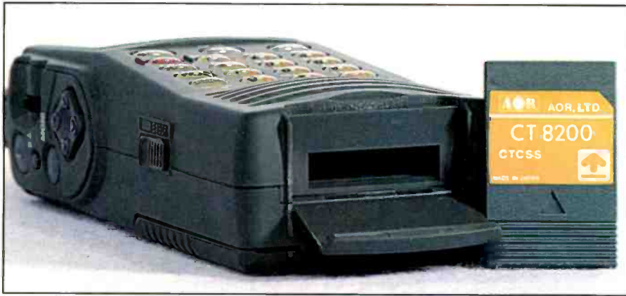
CTCSS used to be optional even on the high-end receivers. The AOR AR-8200 requires an external card be installed for it, as did many early Uniden models. And they weren't all that easy to install, either.
