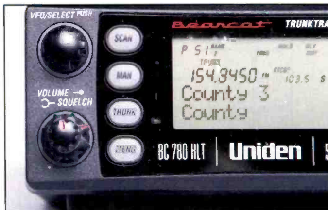
Many of today's trunktracking scanners also feature CTCSS and/or DCS decoding. Here the tone appears to the right of the frequency.
