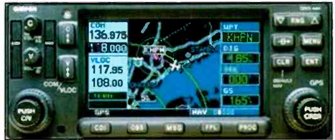
The Garmin GNS430 is an aviation radio that combines ILS, GPS, and VHF voice communications in one handy package.
