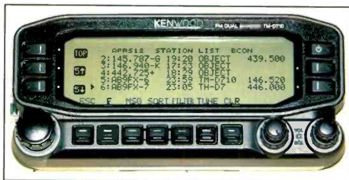
The screen of the TM-D710 transceiver from Kenwood displays APRS objects as they are received. (APRS website photo)
