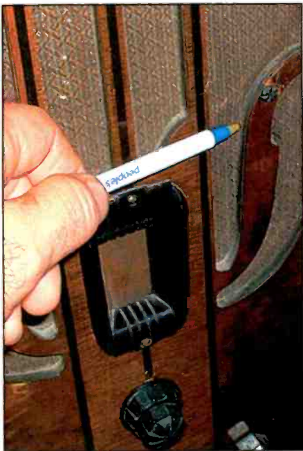
Photo B. I'm using this handsome Philco 44 tombstone to show two points made in the column. First, notice the narrow fretwork and decorative screw head the pen is pointing out, one of four screws used to mount the heavy speaker assembly to the cabinet. Also, the Bakelite escutcheon on this radio is very similar to the 16B tombstone escutcheon that was smashed during shipment.
