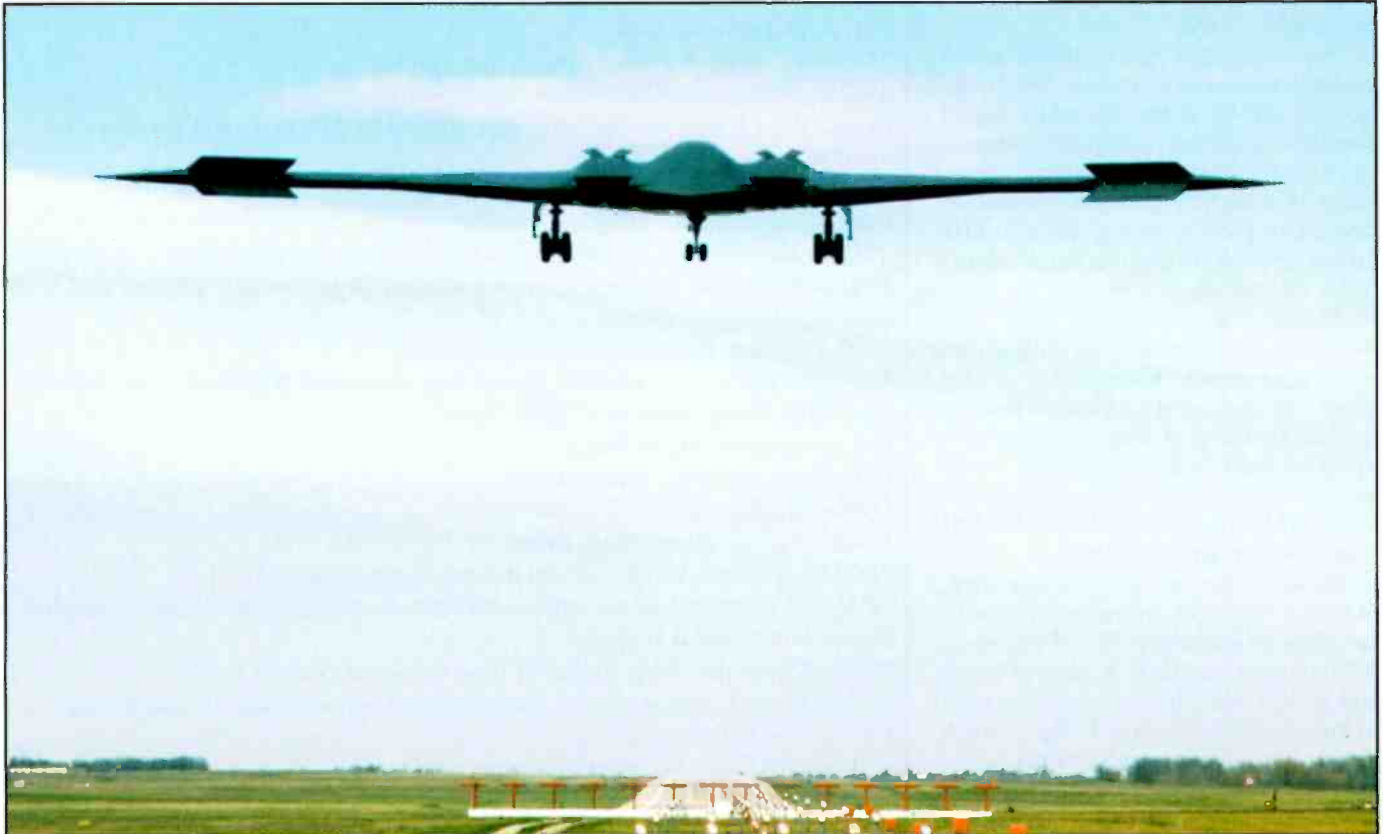
A B-2 bomber landing at Whiteman AFB. The localizer antenna array is visible below the aircraft, at the end of the runway.
