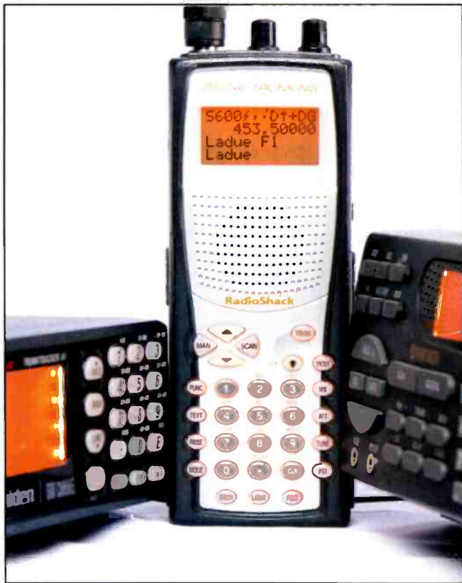
Trunktracking scanners are now available in all shapes and sizes and a few include digital modulation as an option.
