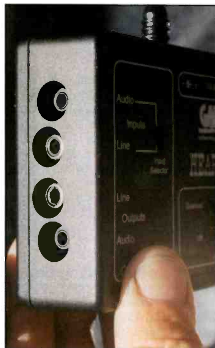
The GAP in-line DSC module with multiple inputs and output jacks.
