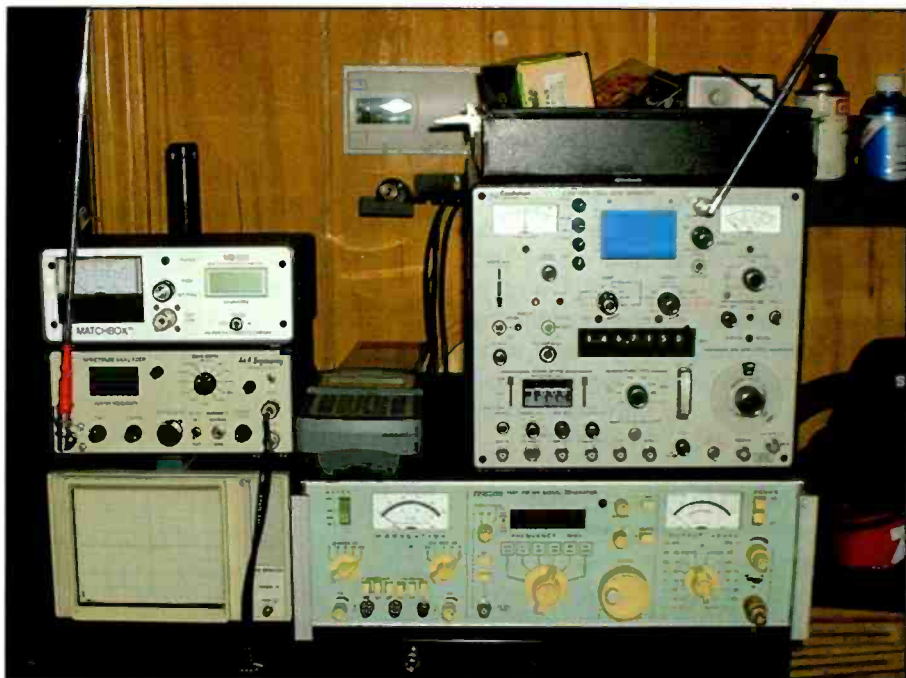
Photo B. My Boonton 102F generator. The modern-looking unit above it is a Cushman model CSM-50A cell site monitor; its features include a signal generator, spectrum analyzer with tracking generator, and a receiver that can accurately measure AM modulation percentage, FM deviation, and frequency. These service monitors are commonly used for aircraft, marine radio, and commercial two-way radio servicing. Their prices are falling and they're becoming a bit more affordable. The Tektronix X-Y display scope is a spectrum display for a highly modified A&A Engineering spectrum analyzer.
