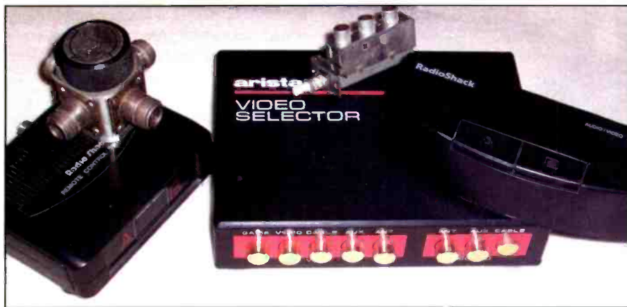
Photo C. TV antenna and video and audio switches you can use to switch SWL antennas.
