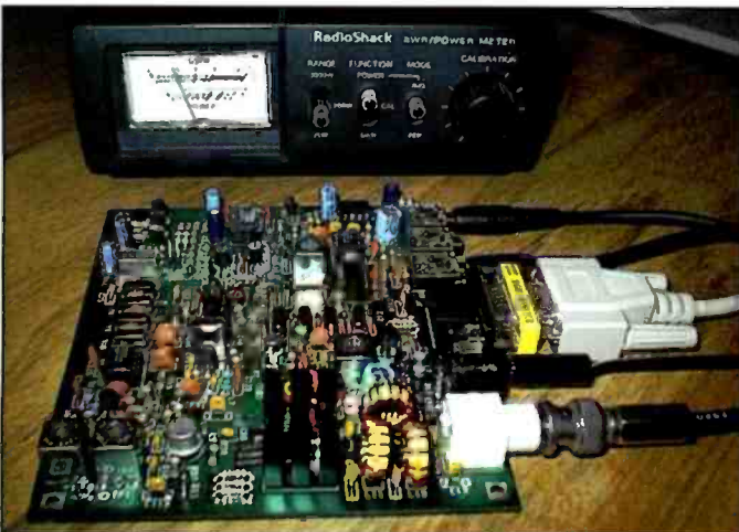
Want to make your own PSK rig? I don't mean just the sound and I/O interface—I mean the entire PSK31 transceiver! Thanks to the kits that are available from Small Wonder Labs, you can build a complete PSK31 transceiver for 20, 30, or 40 meters for about $100 (about $60 for the new 80-meter version). The 20-meter model is shown here. It runs on 12 Vdc and puts out 2–3 W—enough to make stateside and DX contacts, especially on 20 meters. See all of the versions at www.small-wonderlabs.com . This photo is from K1VY's excellent PSK page at www.psk31.com .
