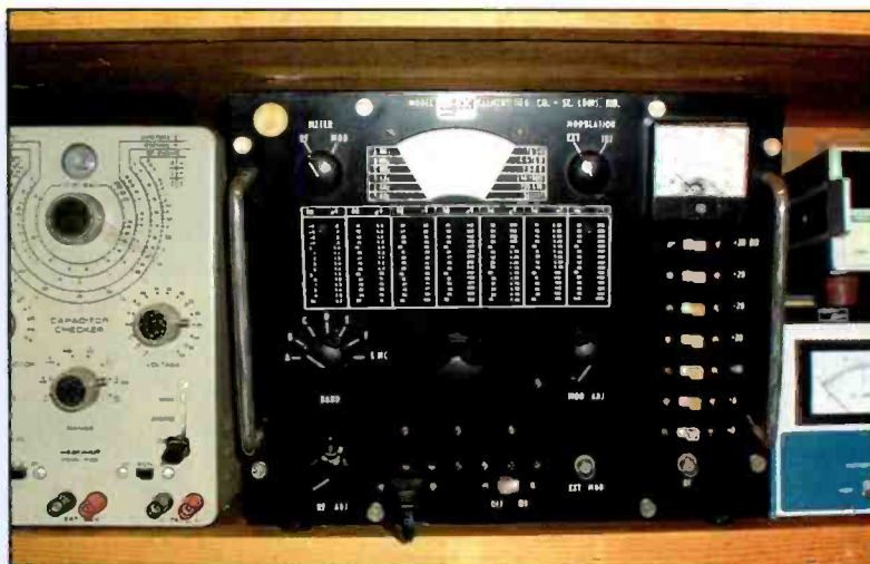
Photo C. This is one of the two Clemens signal generators I own. They're very basic units, but have lab-quality features. They have decent analog dials that are accurate and precise, they're stable, and the RF signal output level attenuator setting is accurate. Also the percentage of AM Modulation can be set to the desired level. These last two features are needed to do accurate Signal-Plus-Noise-to-Signal Ratio measurements.
