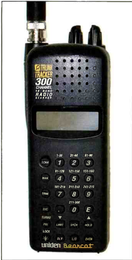
This Uniden Trunktracker was greeted with great enthusiasm when it first appeared. Prior to this, there was no easy way for a scanner listener to follow along with the conversations on a trunking system.
