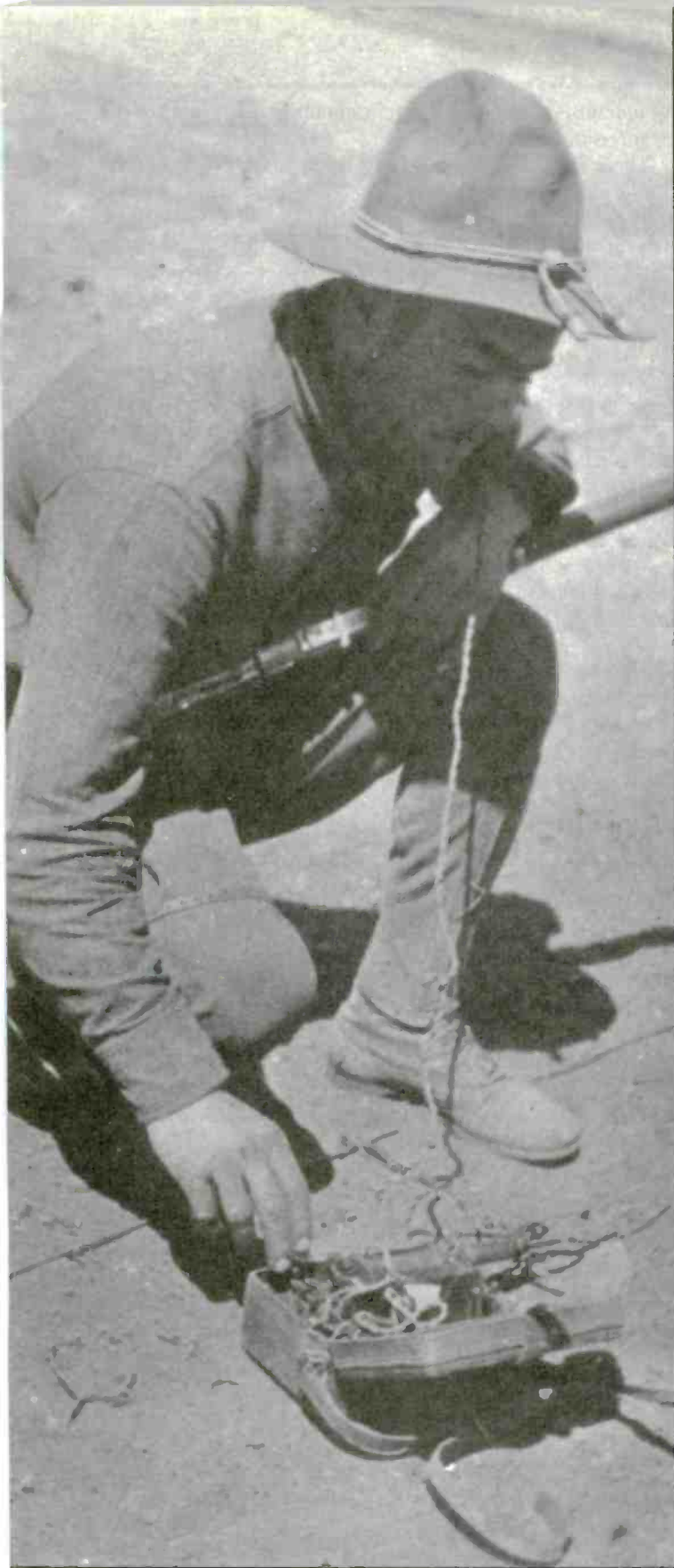
Sergeant William M. Ford operating a model 1914 EE63 Service Buzzer during the Pancho Villa Campaign in Mexico in 1916. Ford was the southernmost Signalman during the campaign. The buzzer, built by Western Electric, was strictly a portable instrument issued to troops in the field for use with all kinds of communications. (Photo courtesy of the Fort Huachuca Museum, donated by William M. Ford)
