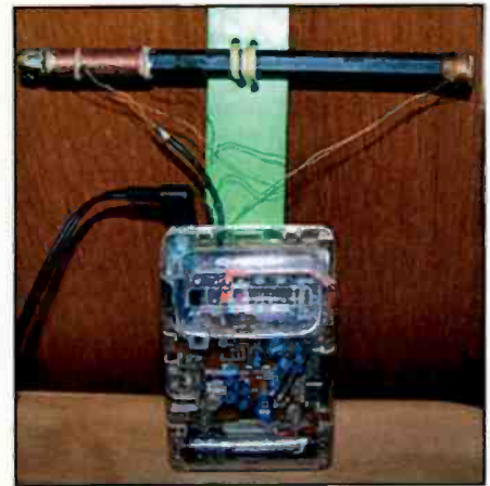
An unlimited class SRF-39P ultralight with hardwired external ferrite loopstick modification by Gary DeBock.
