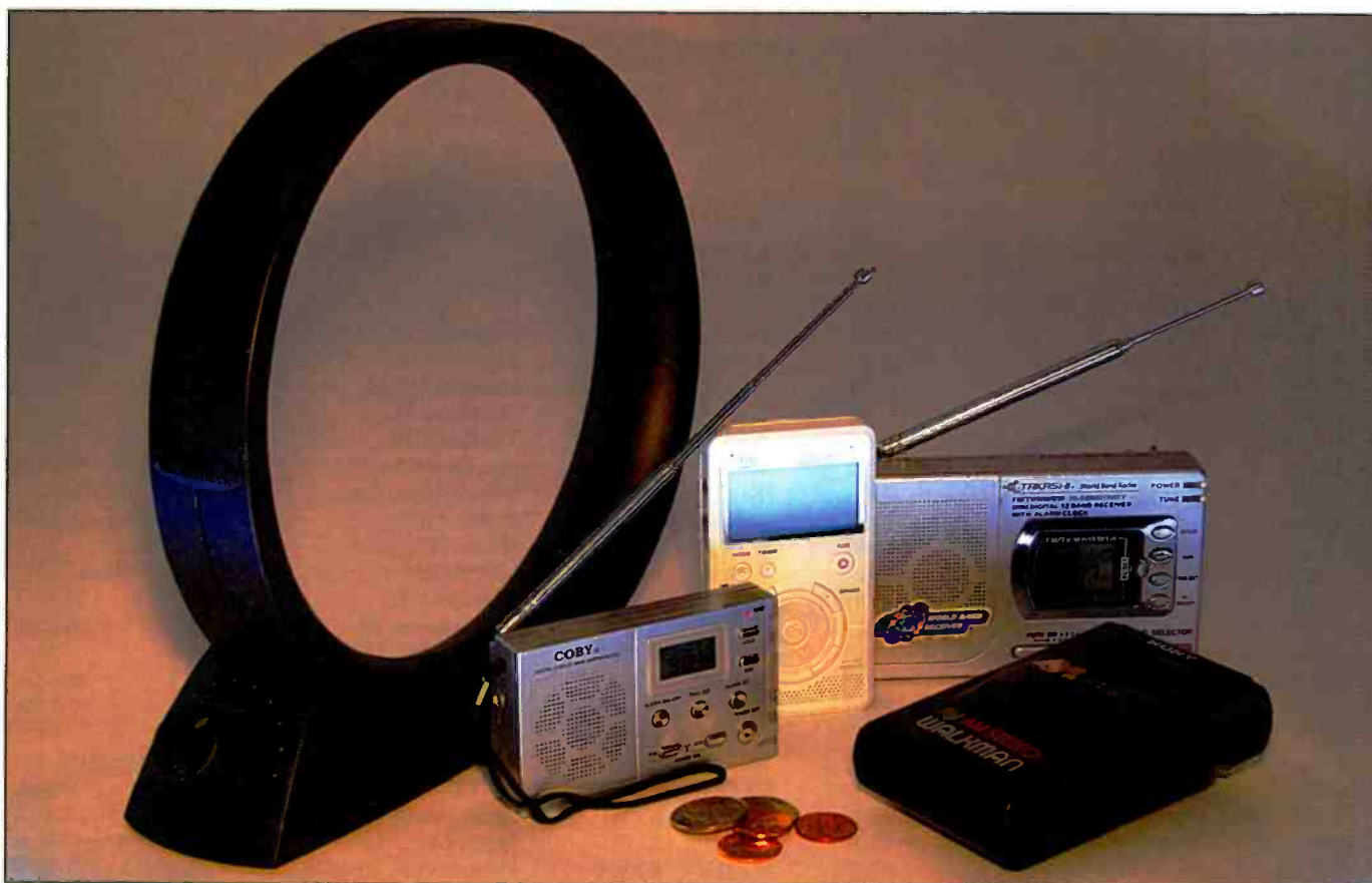
Reception on ultralights like the Coby CX53, Pogo Radio Your Way LX, Takashi World Band Radio, and Sony SRF-42 AM Stereo Walkman can be enhanced by the RadioShack AM Loop or similar inductively coupled loop antenna.
