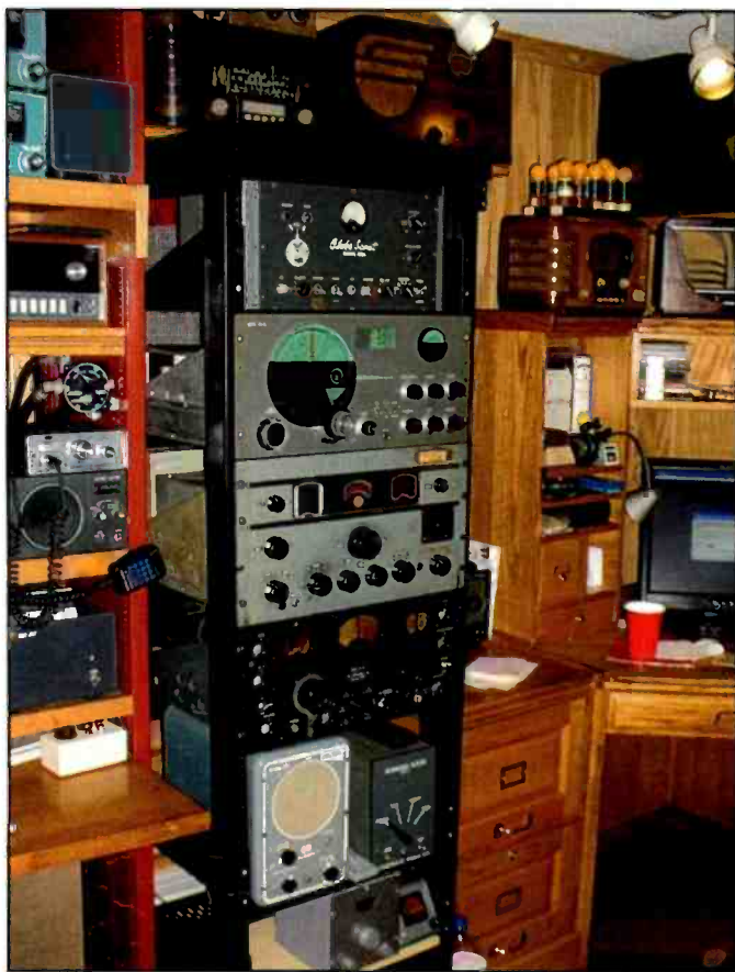
Photo A. This rack is full of "heavy metal" vintage communications equipment and accessories. At the top of the rack is a vintage Globe Scout 40A ham transmitter. Going lower, the large receiver with the modernistic styling (by famed industrial designer Raymond Loewy) is a Hallicrafters model SX-42. The RCA AR-88 receiver (middle of the rack) was exported by the United States to the United Kingdom and the USSR during WWII as part of the Lend-Lease war program. They're scarce in the states, but common and popular in both Canada and the UK. The bottom receiver is a Hallicrafters SX-28, an extremely popular vintage communications receiver from the WWII era with classic styling and a handsome, funky look. The two units beneath the SX-28 are SSB (single sideband) adapters; one is the B&W model 370, the other is the Central Electronics model A Sideband Slicer.
