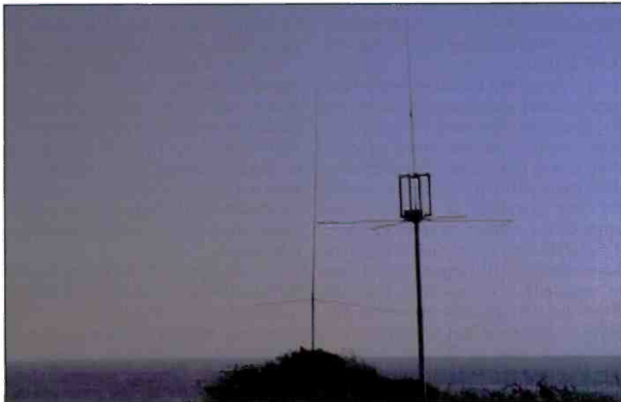
Photo A. Antenna array from the CODAR site at Long Marine Laboratory in Santa Cruz, California. See text. (Photo courtesy of U.S. Navy)
