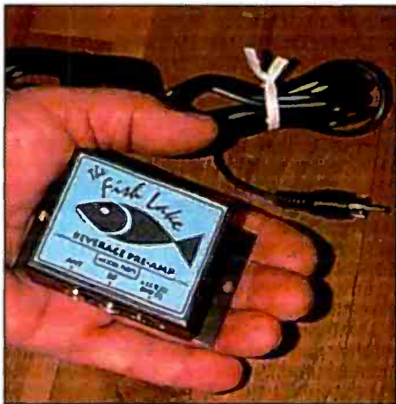
Improve your "ears" on the low bands with the K8LV Fish Lake Beverage FLP1 pre-amp.
