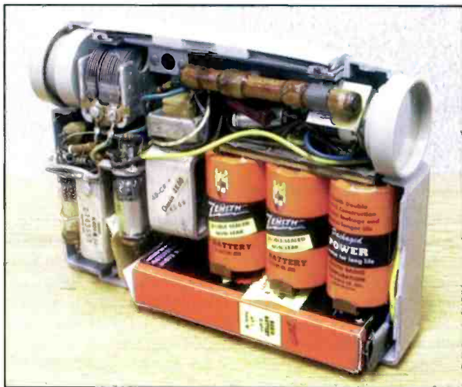
Here are some more examples of Bill Morris' batteries. These are replica Zenith batteries and look quite at home in this vintage Zenith battery personal AM portable.
