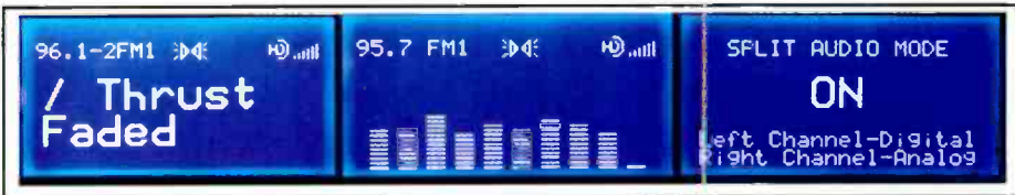
The HDT-1X offers large size text, audio spectrum, and split audio displays.
