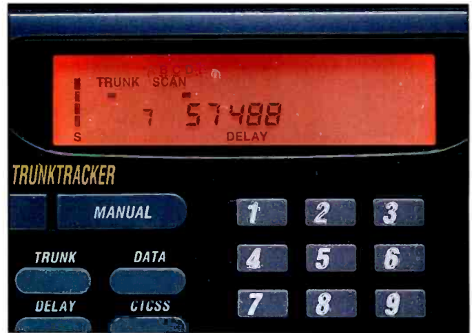
In the trunking mode, scanner banks become sets of talk groups, shown here as A-E. Each talk group is effectively a channel in a trunked system, regardless of how many actual frequencies are involved in the trunked system.
