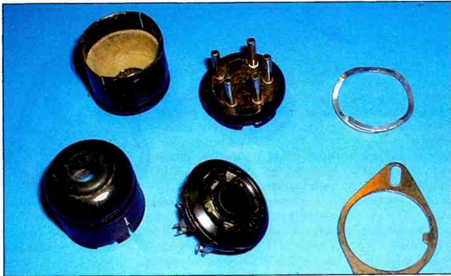
Photo J. These two socket caps, along with an S-type five-pin socket, five-pin plug, and some wire, are the materials needed to construct a speaker extension cable that will let you leave the speaker in the cabinet when testing and aligning the chassis.
