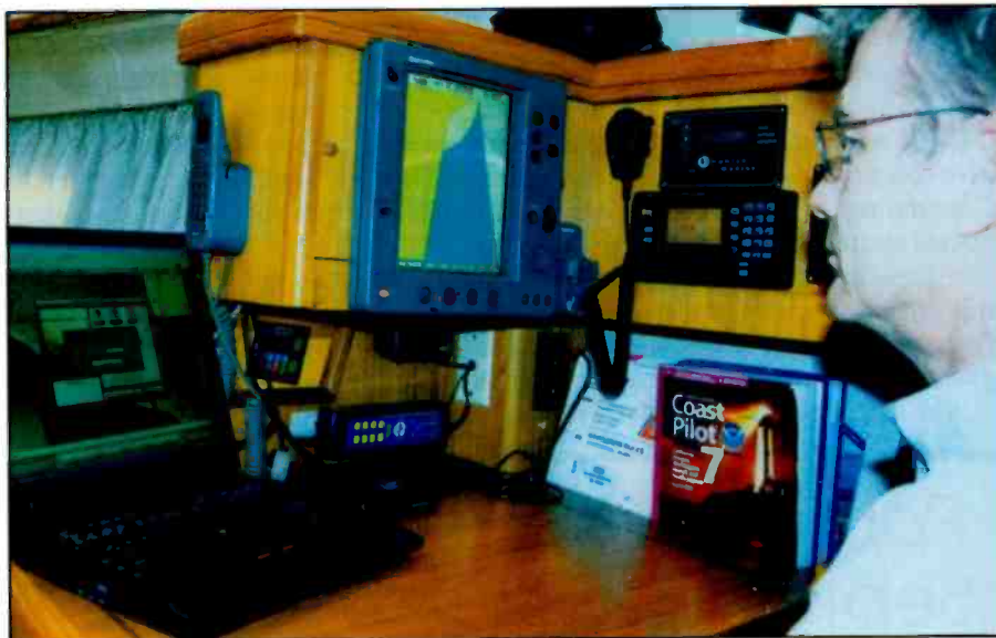
The computer download makes programming the ICOM IC-M802 a breeze aboard a boat.
