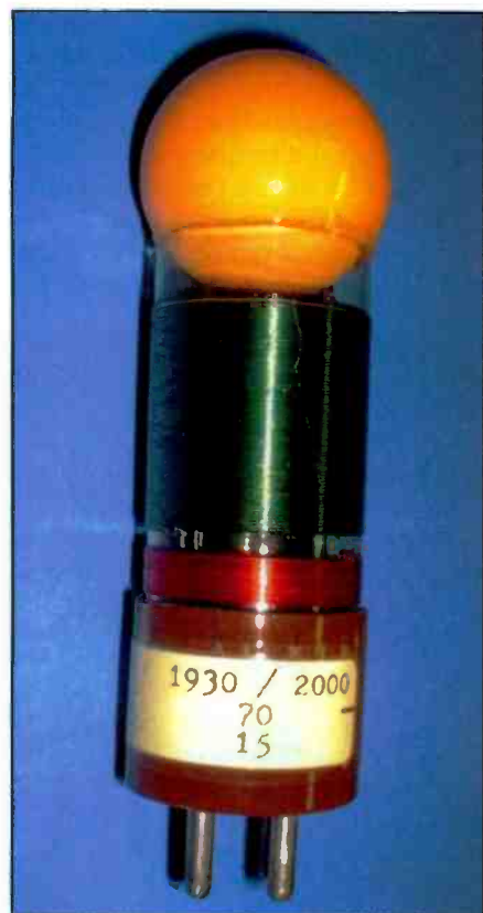
Photo H. Here's another close-up of one of Bob's coils. It looks like it should cover the upper portion of the BCB.
