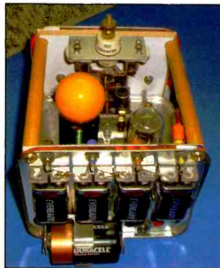
Photo C. Bob included these metal Keystone battery holders on the back apron to supply the filament and B+ voltages. Jumpers allow selecting the detector voltage in 9-volt steps between 9 and 36 volts.
