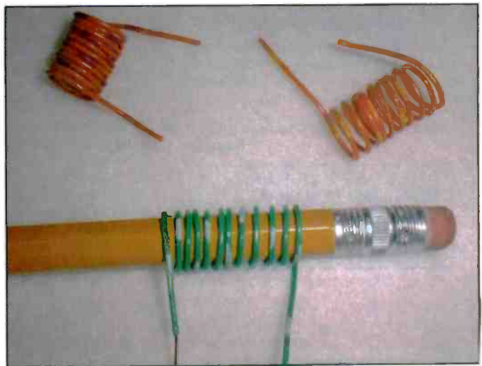
Photo D. Winding your own .47- \mu H inductors.
