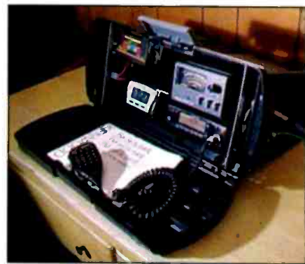
This is the picture that started it all! This Go-Box was fabricated by Steve (KB1DIG) and Kim (KB1GTR) Merrill of Dover, New Hampshire. I stumbled across it on one of my late-night romps across the Internet. Steve and Kim used a file box as the basic container for their portable EmComm radio station. Notice that they've incorporated an SWR meter and power distribution in addition to the basic radio gear. (Photo by Steve Merrill, KB1DIG)
