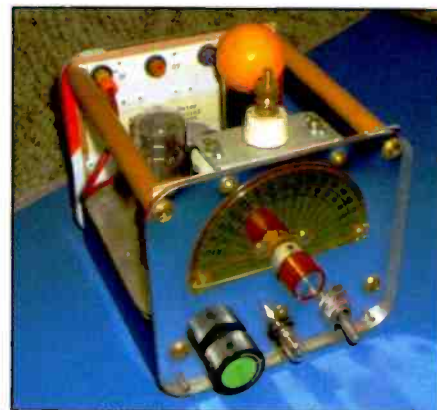
Photo B. A front view of Bob's "Dumpster Diver Special" shows how he's used a protractor for a dial scale and other salvaged materials for the chassis and end plates.
