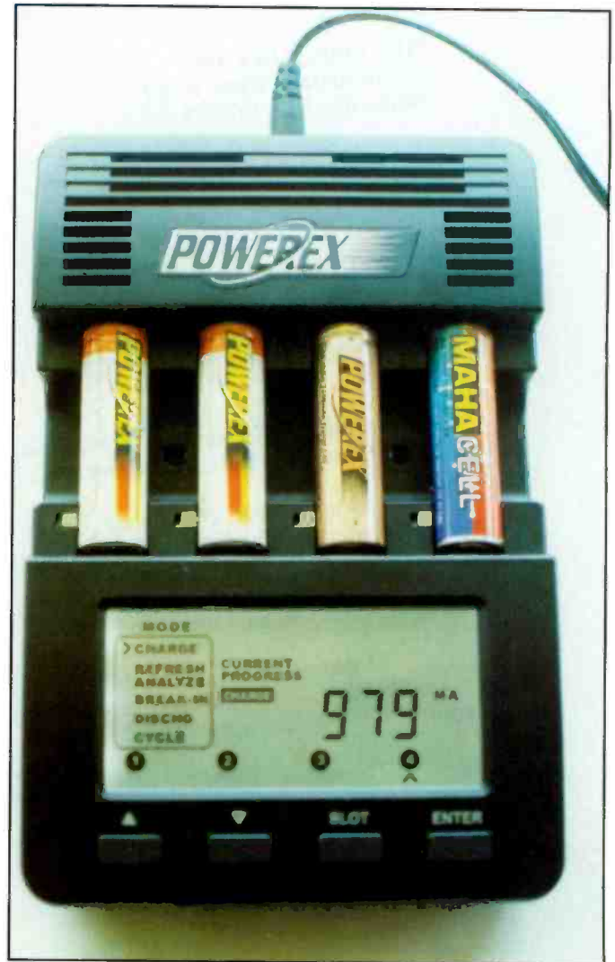
Here the PowerEx MH-C 9000's display shows battery #4 half full, with 979 mA of charge.
