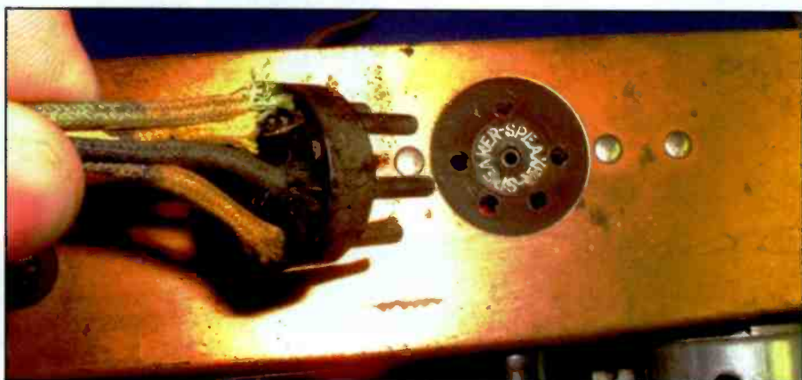
Photo I. Zenith used five-pin wafer sockets for the speaker connection on many of its early console and tabletop radios.
