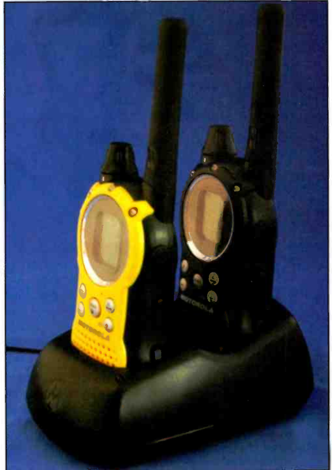
Here's a set of Motorola T-9500 FRS/GMRS handheld transceivers, with NOAA Weather Radio receiver built in, sitting in their standup charger. The radios are furnished with a 3.6-VDC NiMH rechargeable battery pack, but they'll also accept three standard "AA" cells (either alkaline or Lithium-Ion), so you'll have plenty of power if you include an extra set of "AA" cells in your gear bag.
