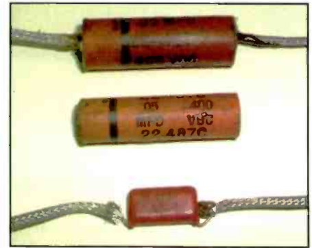
Photo F. Here's a method to achieve the same electrical and mechanical benefits attributed to the early wax bypass caps that incorporated braided wire leads. A modern capacitor is fitted with braided leads made from lengths of 1/8-inch wide desoldering braid. The new capacitor can be hidden in the old cardboard shell that housed the original wax capacitor to maintain the original chassis appearance.
