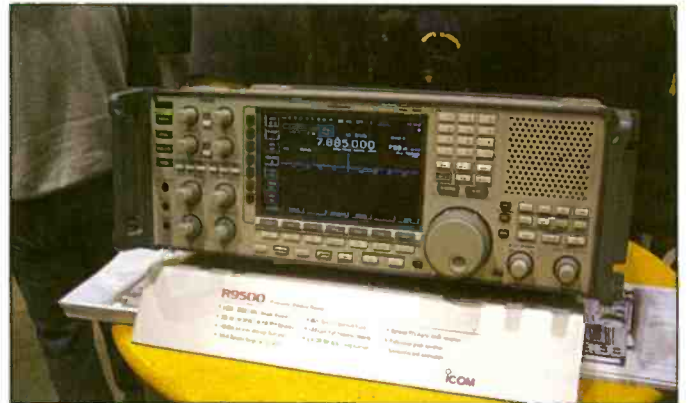
Photo B. ICOM's R-9500 covers 5 kHz to 3,335 GHz. Its peak search function automatically tunes the receiver to the strongest signal on the spectrum display.
