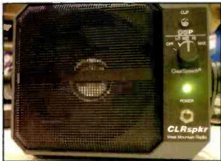
Photo D. West Mountain Radio's CLRspkr is an amplified speaker featuring ClearSpeech digital signal processing. It's designed for mobile or home station use.
