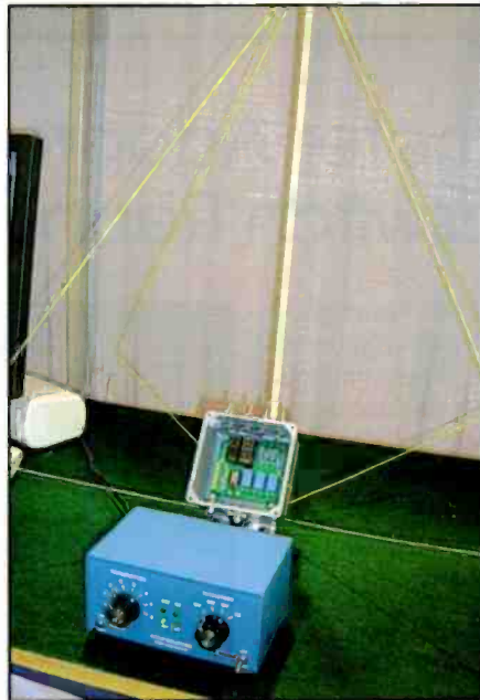
Photo E. This is a scale model of the AS-AYL4 K9AY 4-direction receive antenna from Array Solutions. The real one is 24 feet tall and lets you remotely change receive patterns.
