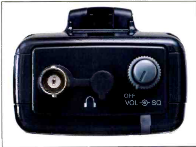
Top view of the PSR-500 showing the BNC antenna jack, earphone jack, and volume/squelch control.
