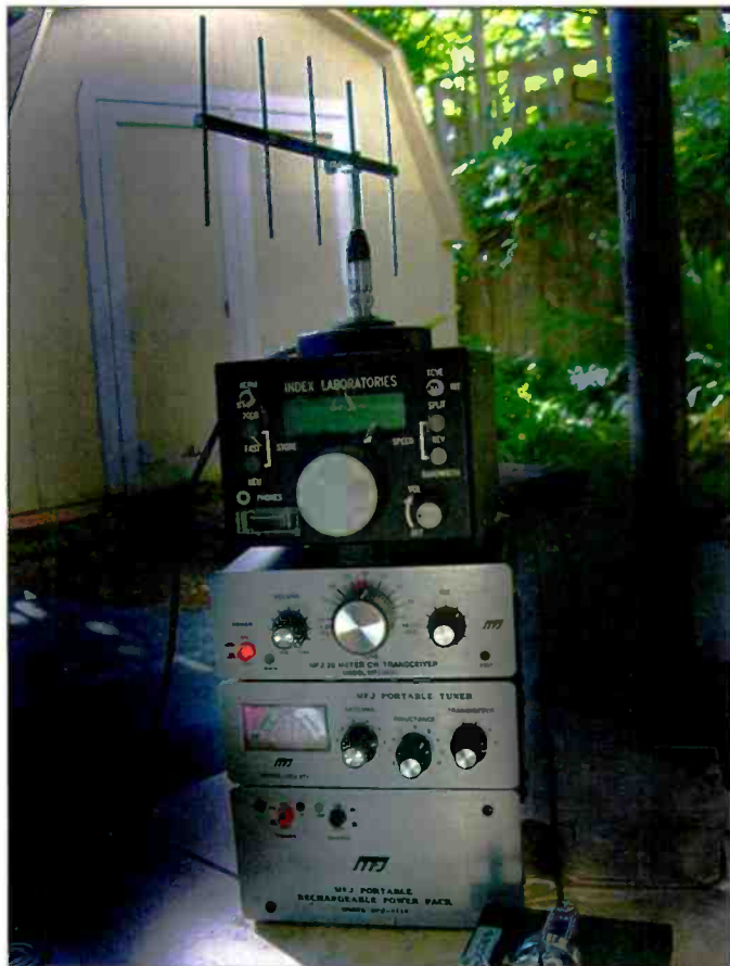
The author's portable HF equipment.
