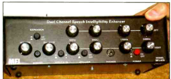
Photo C. The dual-channel speech intelligibility enhancer from MFJ provides a separately tunable output for each ear to compensate for hearing differences from one ear to the other.
