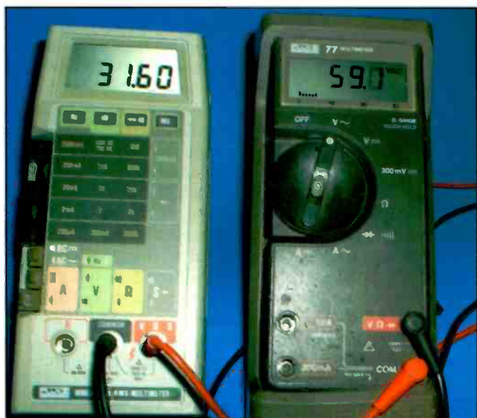
Photo B. These two Fluke meters were part of an experiment that shows how a non-symmetrical waveform, such as is produced by a half-wave rectifier, can affect the reading of a "True RMS Multimeter." Note that the Fluke 8060A (to the left) is displaying 31.60 volts AC instead of the expected true RMS voltage of 41.71 VAC (0.707 x 59.0 volts).
