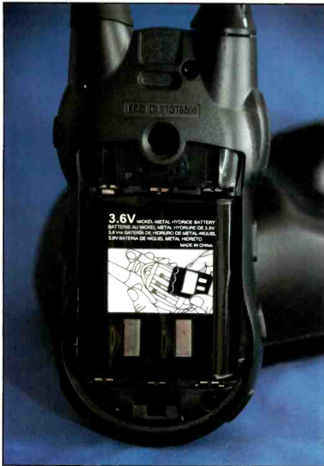
A close up of the rechargeable battery pack loaded into the back of the T-9500 transceiver. These Nickel-Metal Hydride packs offer a higher power density (ability to power the radio over longer periods of time under heavy usage) than the same size NiCad packs. Add a spare set of "AA" Lithium-Ion cells (three total) and you are set. I get my Lithium-Ion "AA" cells at Wal-Mart, as they seem to be the cheapest. A six-pack of Li-Ion "AA" cells coupled with the rechargeable battery pack will last a long time in the bush.
