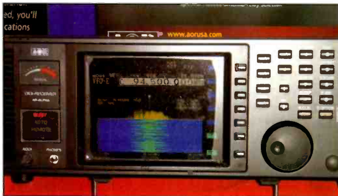
Photo A. The AOR AR-Alpha receiver is a professional-grade receiver covering 10 kHz to 3.5 GHz in just about any mode you can think of (and maybe a few you can't!).
