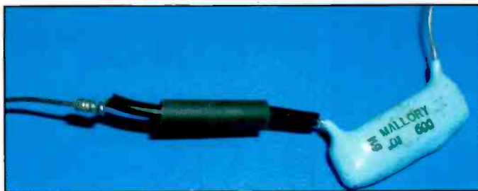
Photo C. Sometimes it's a bit risky to fully remove old component leads from friable, aged Phenolic bandswitches or tube sockets. This simple technique achieves a neat splice, which is also electrically and mechanically sound, to avoid stressing those irreplaceable parts!
