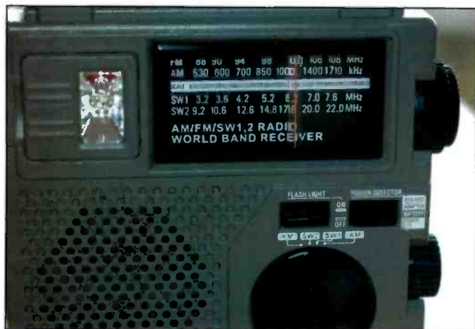
Photo 3 - A close up of the analog display and controls. It's very well laid out and ergonomic. It's not a DXing radio but will definitely bring in local AM/FM and world band SW stations.
