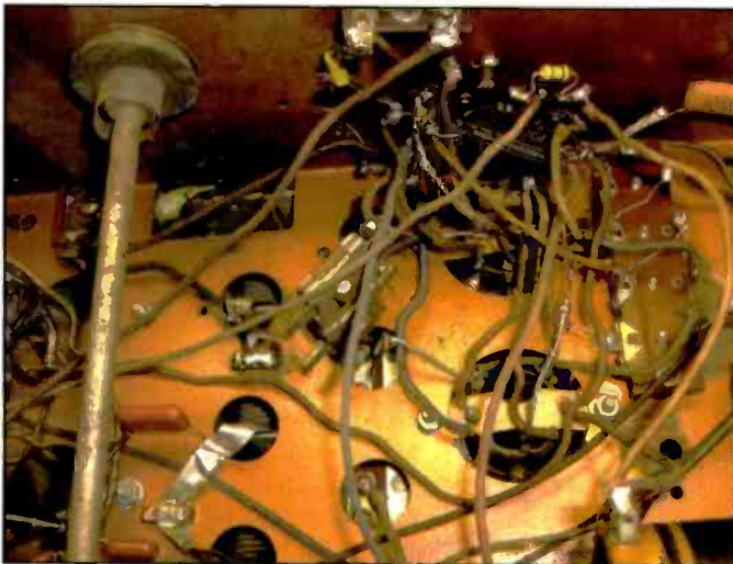
Photo D Fortunately the bandswitch for the 7S232 uses only a single phenol wafer section, but even so an impressive rat's nest of wires interconnects the complex bandswitching used in these early radios!
