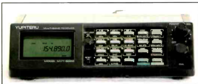
MVT-8000: During the height of the silliness associated with the banning of cellular-capable scanners, many enthusiasts imported receivers for personal use from Europe or Japan. This is a Yupiteru MVT-8000, an excellent receiver that featured full coverage. Its small size made it easy to mount almost anywhere.
