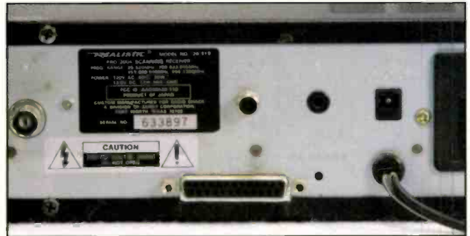
PRO-2004 (rear view): One of the innovations that came out of the 2004 was the idea of hooking it to a computer. The interface was difficult to install for the faint of heart, but it could be done with a bit of patience and a soldering iron. With the interface, the radio could be reprogrammed by a computer in just a few minutes, as opposed to hours of painstaking keypad entries.
