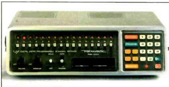
PRO-2001: In the late '70s Radio Shack and Bearcat both had a number of breakthrough receivers. This is the first digital entry model that I was aware of then, although Bearcat had some out prior to this one. It had sixteen channels, but the keypad allows for direct entry of the frequency.
