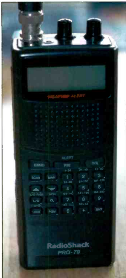
Photo 4 - My old faithful Radio Shack PRO-79 that I picked up on closeout sale a few years ago for under $100. This is a nice little 200 channel conventional scanner. It WILL NOT track or decode analog or digital trunked systems, which is not a problem in my area. Pick your hand held scanner carefully, look for sales and spend your money wisely; your safety and that of your family's might well be at stake.
