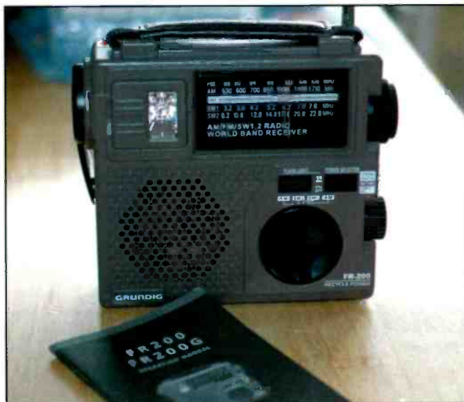
Photo 1 -This is a shot of the front of the FR-200 Grundig "survival" radio. Nice, clean, functional, AND analog! Radios with digital displays hog battery power while an analog display doesn't.
