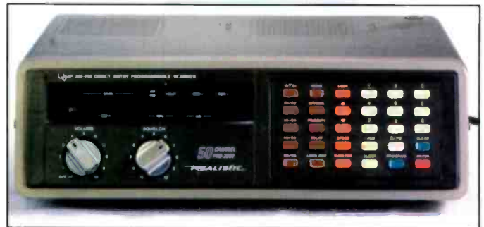
PRO-2002: Not to be outdone, Radio Shack quickly offered a product with 50 channels as well. Instead of the service search function, this was the first scanner that had search ranges (more than one!) that could be programmed. The S1-S5 on the banks switches represent search ranges that could be enabled or disabled.
