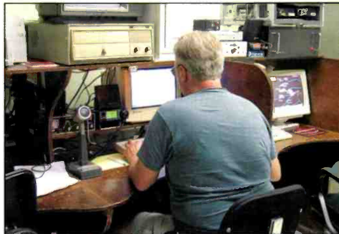
N2WUT operating a station at the EOC during a 2006 disaster preparedness exercise. An APRS display for tracking vehicles by radio can be seen on the computer monitor at right.
