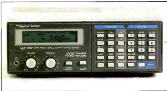
PRO-2005: The PRO-2004 quickly gave way to the PRO-2005 (shown) and later the PRO-2006, which looked virtually identical. These receivers were the mainstay of the scanner world for a long time. Sporting 400 channels combined with an efficient receiver, and later with the availability of computer control, made this a hard combination to beat. Then the Electronic Communications Privacy Act of 1986 made it illegal to manufacture and sell a receiver that received or could be easily modified to receive cellular frequencies. But on the PRO-2006 you only had to snip one diode to get them, so the receiver was discontinued. They can still be found on eBay, however, and command a premium price with some scanner enthusiasts.
