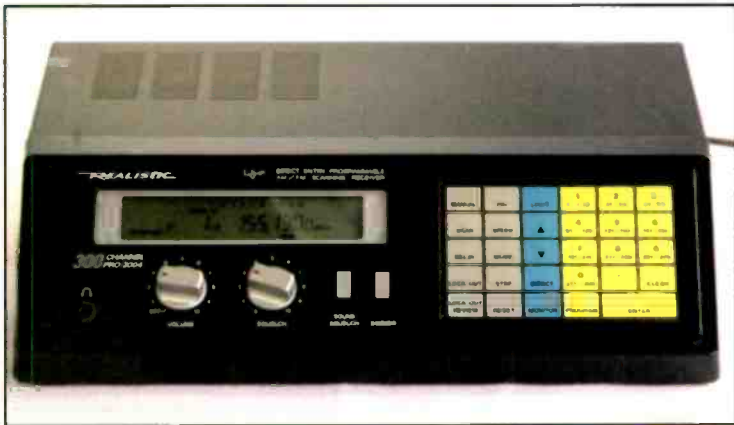
PRO-2004: This represented another major innovation: 200 channels, as opposed to the 16 or 50 that were common. The 2004 was also the first scanner to lend itself to modifications of the circuit by "hackers."
