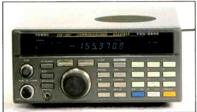
FRG9600: All of the major ham and commercial radio manufacturers also made communications receivers that covered the VHF/UHF range. The Yaesu FRG9600 was one of the first that came from the factory with a built-in computer interface, although software was nowhere to be found until ScanCat came along. This is an excellent receiver, but a terrible scanner without computer control. Coverage on the FRG9600 is continuous, but starts at 60 MHz, leaving out the VHF low band completely.
