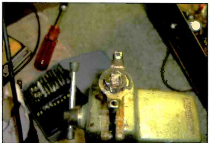
Photo G Here's a good view of the end of the shaft where the device that drives the switch wafer is attached. The repair involved drilling and tapping the shaft so a 4-40 screw could be used to hold the assembly together.
