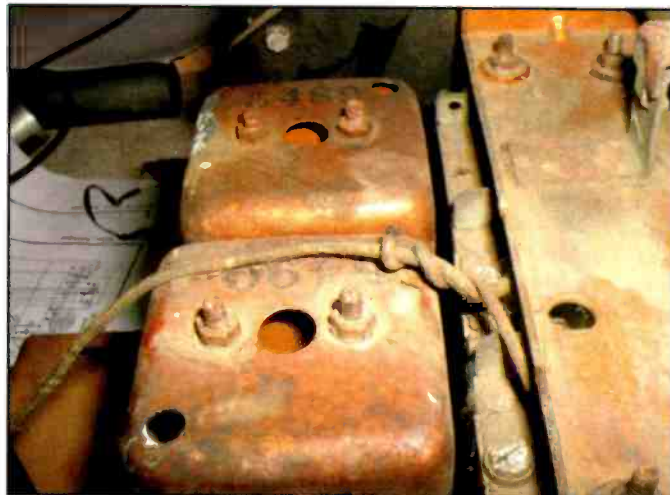
Photo B. Twisting two short lengths of insulated wire together can make a quick, inexpensive low value capacitor. These are called "gimmick capacitors" in the trade.
