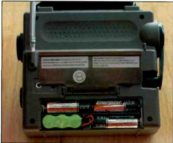
Photo 2 - Here is a shot of the back of the FR-200 Grundig "survival" radio. Note the green bundle of small cells on the bottom left: these are the NiMH rechargeable cells. These cells can be recharged by an external 4.5 V DC wall-wart or using the crank generator on the side of the radio. The three "AA" alkaline cells are shown above the NiMH pack.
