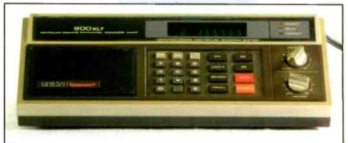
BC800XLT: Another breakthrough happened with the introduction of this device. For the first time a scanner covered the 800-MHz public safety bands. Prior to that time, an agency on 800 MHz was virtually immune to scanner listening.
