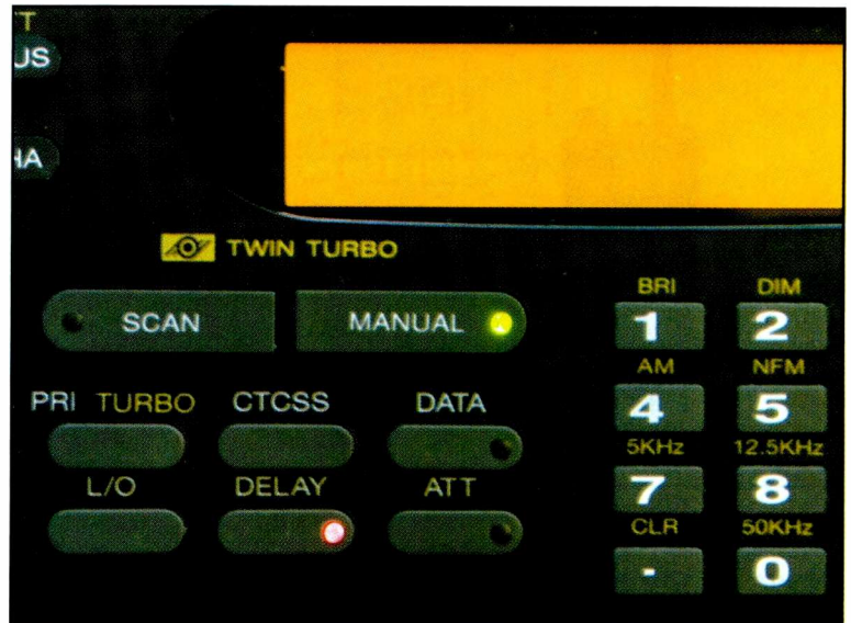
This BC-9000 features a CTCSS decoder, but not DCS. There are still a lot of systems where this is useful and it sure cuts down on interference.
