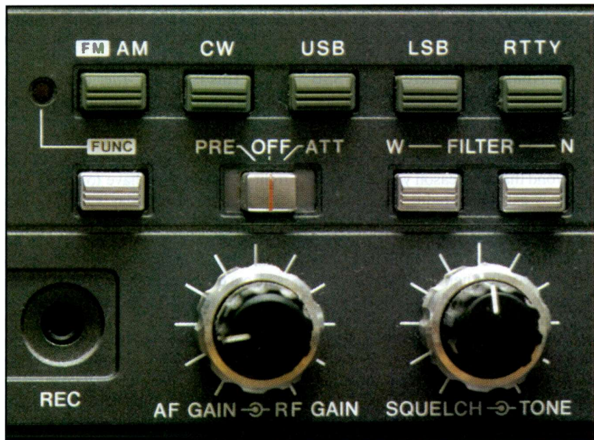
This shortwave communications receiver has the AF and RF gain adjustments located on the same control. The collar is the RF gain, and the front part of the knob is the AF, or volume control. Also note the switch right above this knob which controls Preamp, Normal or Attenuator, but it's all or nothing.
