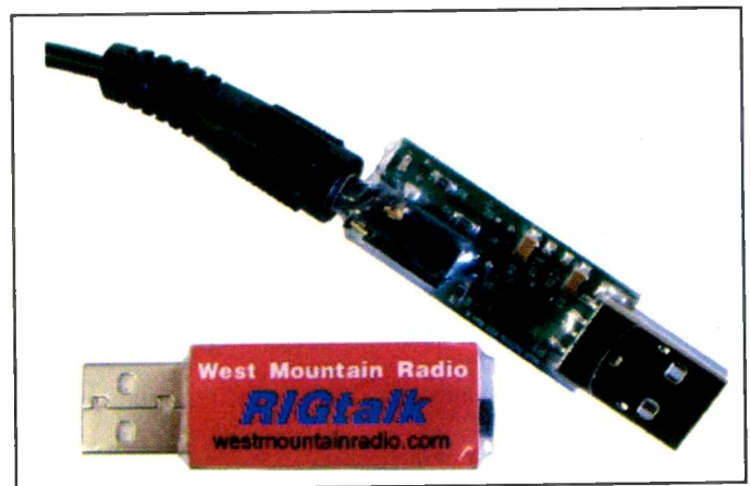
Photo C. The RIGtalk radio-to-USB interface. (Courtesy of West Mountain Radio)
