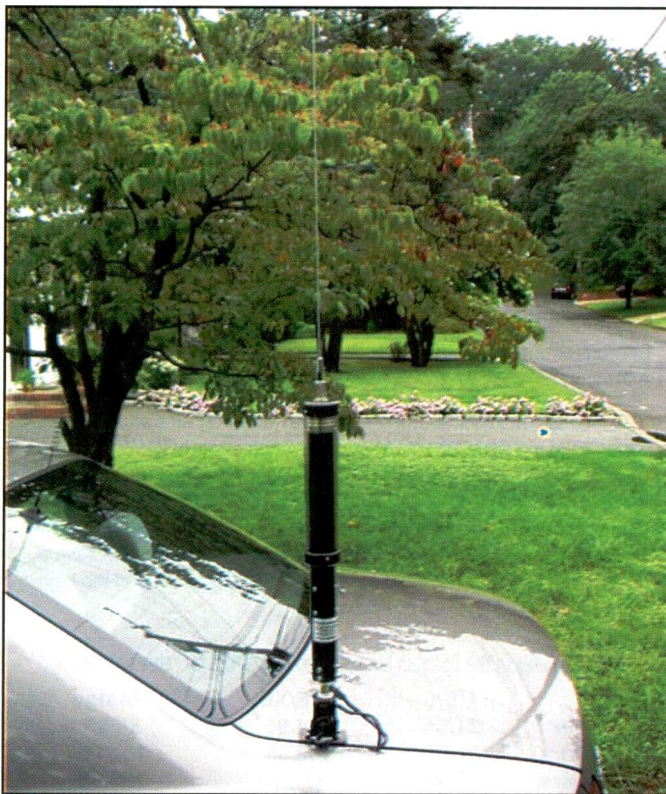
Here's the Little Tarheel II mounted on the trunk deck of our vehicle using the MFJ-348T. The antenna not only looks good, it's a great performer and ideal for mobile SWLing/DXing and even CB!
