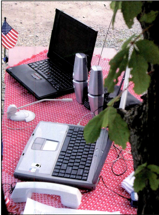
Here's a mock-up of the system that transmits voice data at between 400 and 600 wpm between computers using RemComm's advanced voice recognition software. The system is extremely reliable, usable over any form of radio system, and can be used to link various radio systems together. Goodbye "interoperability problems."
