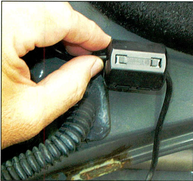
The ferrite core must be placed on the control cable to keep antenna motor noise down during tuning. It also decouples the control wire from antenna.
