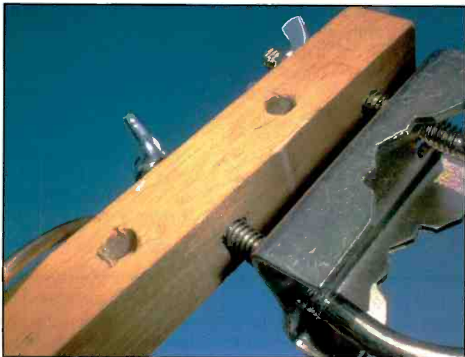
Photo C. U-bolt mounting and wing nuts.
