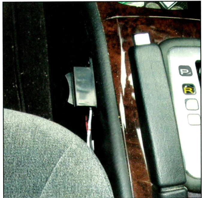
The control switch mounted for easy access. Push to raise or lower the antenna.
