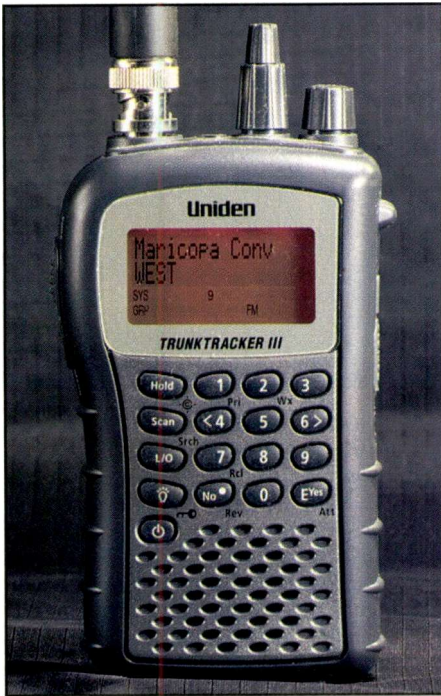
Trunking capability is probably the second decision you should make about a radio you intend to purchase—right after the handheld or base/mobile purchasing decision. This Uniden Trunktracker III represents the latest generation of trunking scanner, but does not cover digital or military air. There's always a tradeoff.
