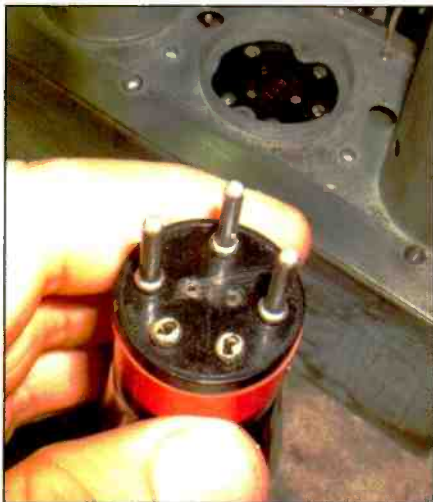
Photo C. A 27 tube is prepped by cutting the pins so it can be used as a dummy tube for neutralizing the RF stages. The tube filament is disabled; this permits neutralizing (balancing out) the internal tube capacity to prevent unwanted feedback and self oscillation. Another possible method would require temporarily removing the B+ from the stage being neutralized, but this difficult to do in the Majestic 90.
