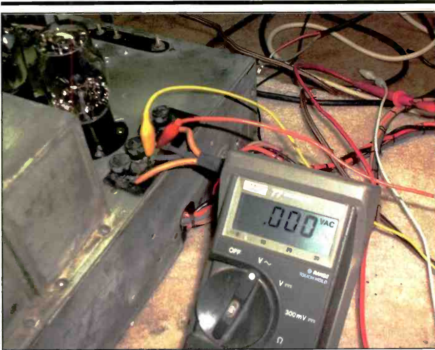
Photo A. A sensitive AC voltmeter is used to monitor the speaker audio during alignment.
