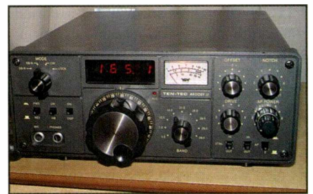
The Ten-Tec Argosy-II is a 5/50-watt output HF transceiver featuring a digital readout. This is a 20-plus-year-old radio, but it's a solid performer even by today's standards. Used prices range from $250 to $350, depending upon options and condition.
