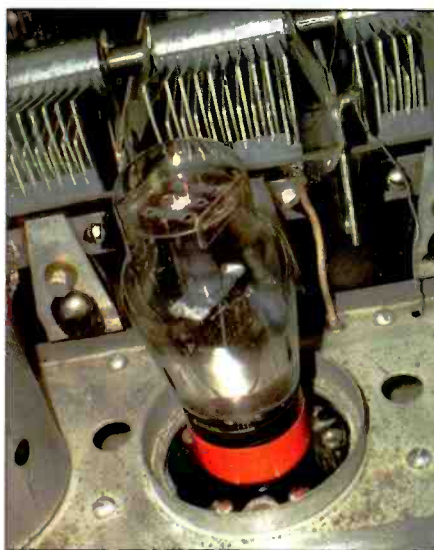
Photo D. The modified 27 dummy tube in use.
