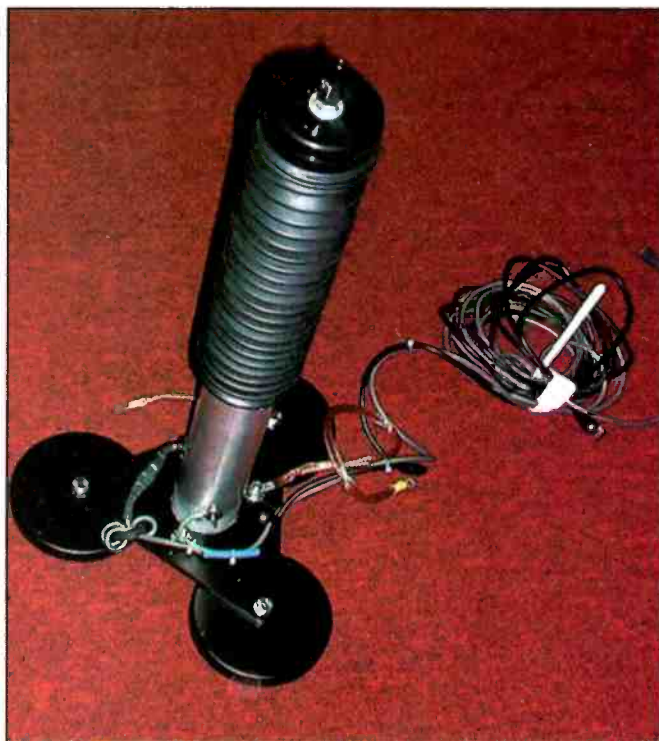
Photo C. The Shorty I and MFJ-336 magnetic mount ready for installation on the vehicle.
