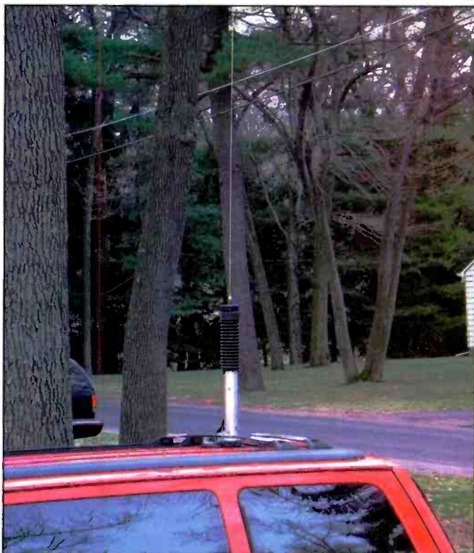
Photo F. I mounted the Shorty I near the rear hatchback on my Voyager van. The center of the roof would have been a better location, but it was inconvenient.
