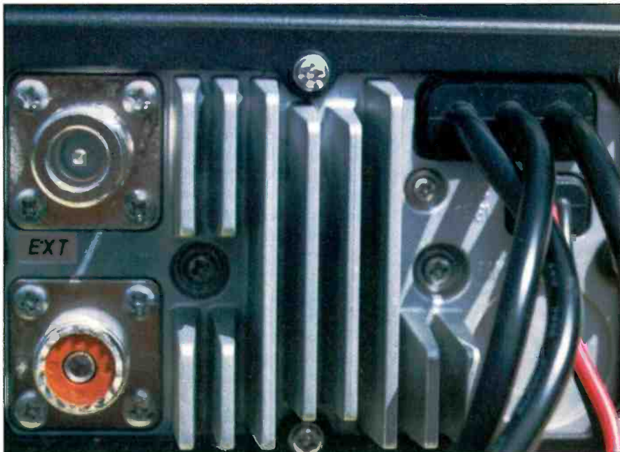
The 2.4-GHz antenna is built in, plus there's a provision for an external antenna (upper left jack).
