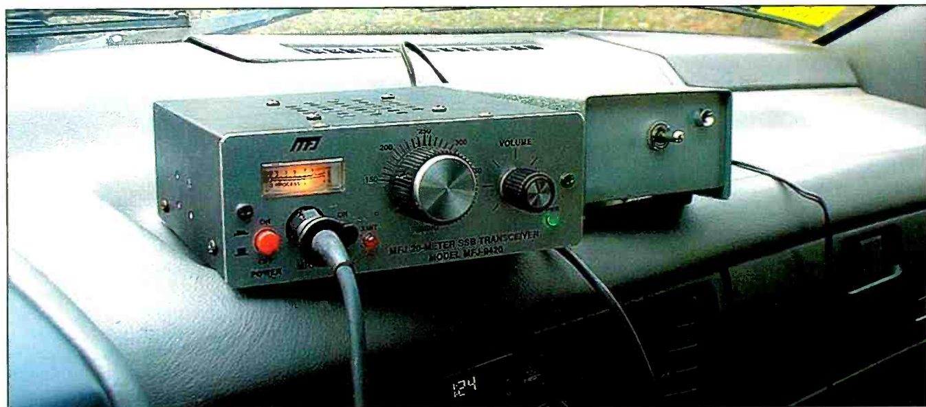
Photo J. My QRP mobile test setup used the MFJ-9420 20-meter SSB transceiver. Worldwide communications are possible when conditions are favorable.
