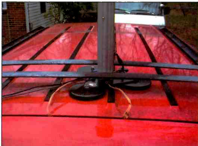
Photo G. I ran the ground straps between the hatchback and van body to the metal body inside the van. Adding heatshrink tubing or tape over the braid will help protect the vehicle paint at the entry points.
