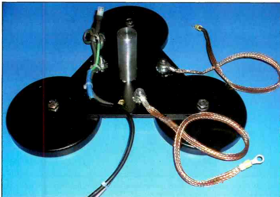
Photo B. A MFJ-336 magnetic mount was modified to allow installation of the Shorty I mounting pin. The antenna can be removed from the magnetic mount by loosening a setscrew and lifting the Shorty I off its mounting pin. Braided copper ground straps are needed to bond the antenna to the car body, which serves as the ground counterpoise for the antenna to work against.
