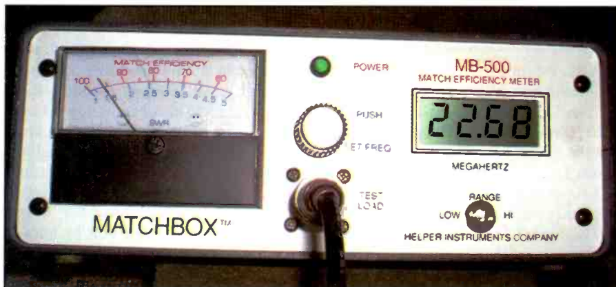
Photo H. A Helper Matchbox proved useful to quickly verify the frequency coverage and SWR across the antenna's advertised operating range. It passed with flying colors!
