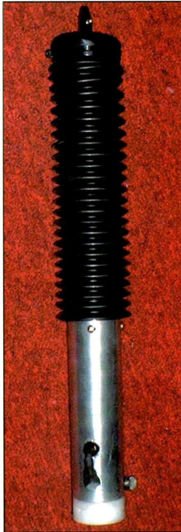
Photo A. Here's the Shorty I antenna. Hidden inside is a remote-controlled DC motor that tunes a variable inductor, permitting the antenna to operate continuously across the HF spectrum! The antenna is well made and very rugged. A stainless steel whip is needed, as well as a means to mount the antenna on your vehicle.
