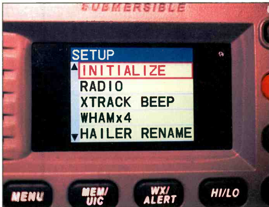
The radio can take up to four "WHAM" 2.4-GHz microphones.
