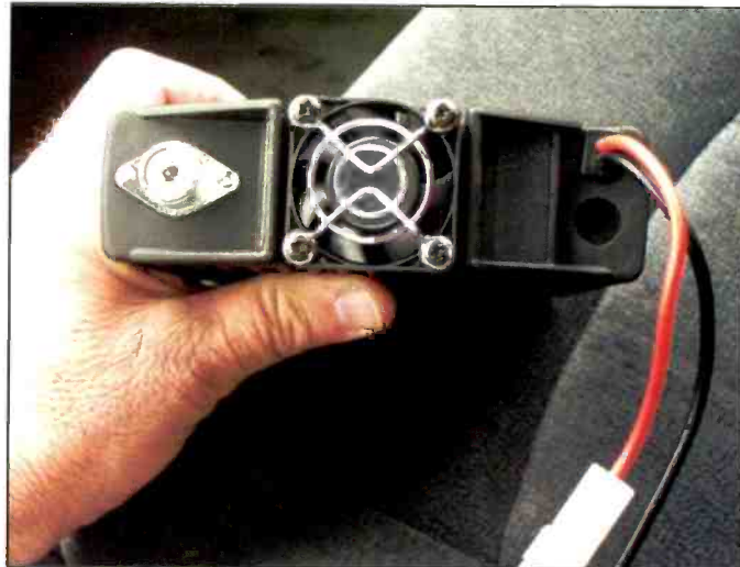
The rear of the 635T showing the perfectly adequate cooling fan.
