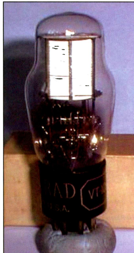
To give those of you who haven't worked with vacuum tubes an idea of what was inside SIGSALY, here's a photo of a model 2051 Gasc Tetrode Thyatron vacuum tube. There were 384 of these inside of one terminal. Imagine how hot the equipment must have gotten when they were all working!
