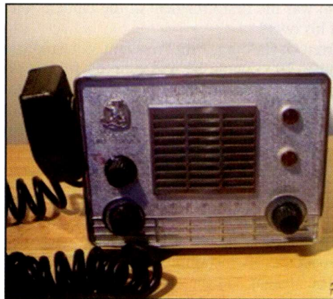
Here's the EF Johnson Messenger One, offering 5 watts input power and five crystal-controlled transmit/receive channels. With its superhet receiver it can easily be converted to 10-meter AM by replacing the channel crystals and retuning the radio. (Courtesy www.retrocom.com)
