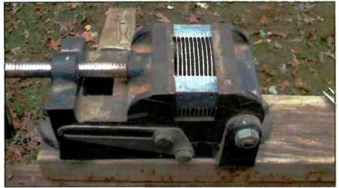
Photo I. Once the pot metal is heated and softened, work must progress quickly before it cools. The machinist's vise was an ideal means to compress the metal. The jaws of the vise assured that pressure was applied equally, and in parallel, to the sides of the blocks. Be sure to use gloves when handling the hot metal parts.
