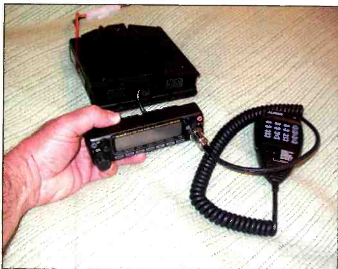
The control head separated from the main body; we'll have more on that aspect in an upcoming Pop'Comm !
