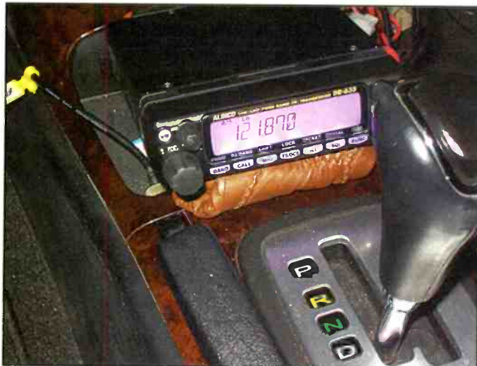
It's a fairly snug fit in our vehicle, mounted on the angled end of an old plastic car vac and a small piece of fabric.
