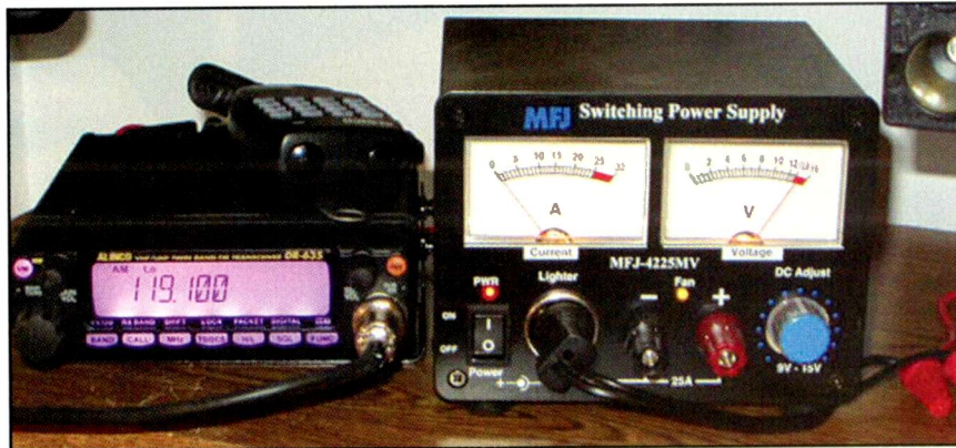
Here's the 635T as a base radio. In this case, I used it as a receiver to monitor nearby Newark International Airport. My power supply of choice is the excellent MFJ MightyLite 4225 MV switching power supply. This compact, lightweight power supply is a great companion to the 635T, offering 25-amp max current (22 continuous) with dual lighted meters
