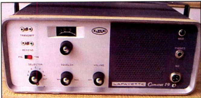
Here is another vacuum tube CB in my basement. Eventually this one will be converted to 10-meter AM along with my EF Johnson Messenger One. These old rigs are great projects for the intermediate builder/homebrewer—not too complicated but enough of a challenge to be a lot of fun. The end result is a good radio on a useable band that won't fold up if there's a nuclear detonation. (Courtesy www.retrocom.com )
