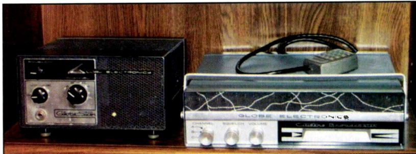
This is a picture of the ECI Courier 23 vacuum tube crystal controlled CB base station (left). An early crystal-plexed synthesizer, it will take a major effort to convert it to 10-meter AM. This unit is exactly like the one I used in college in the mid to late '60s. The Globe Star (right) is another great candidate for conversion to 10-meter AM. This rig is built like a tank.
