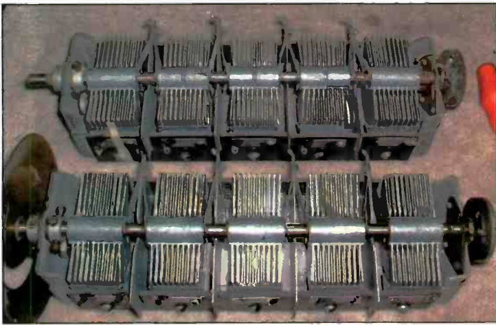
Photo G. Thanks to the kind efforts of two other fellow restorers, these two tuning capacitors were donated for needed parts.
