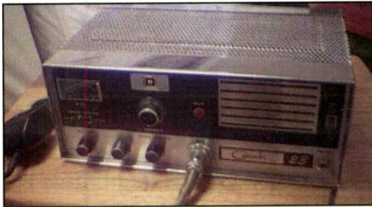
This is a picture of the ECI Courier 23 vacuum tube crystal controlled CB base station (left). An early crystal-plexed synthesizer, it will take a major effort to convert it to 10-meter AM. This unit is exactly like the one I used in college in the mid to late '60s. The Globe Star (right) is another great candidate for conversion to 10-meter AM. This rig is built like a tank.
