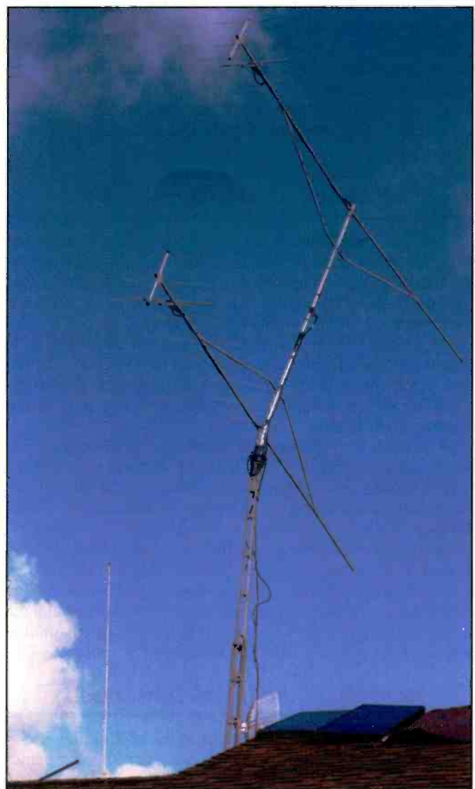
The Tailtwister rotor survived, but the mast couldn't hold up to the 80-mph twister.
