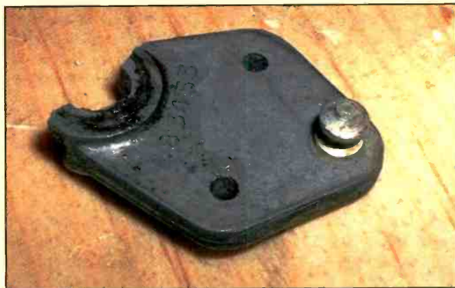
Photo B. The original pot metal linkage arm for the shutter indicator had broken and could not be repaired.
