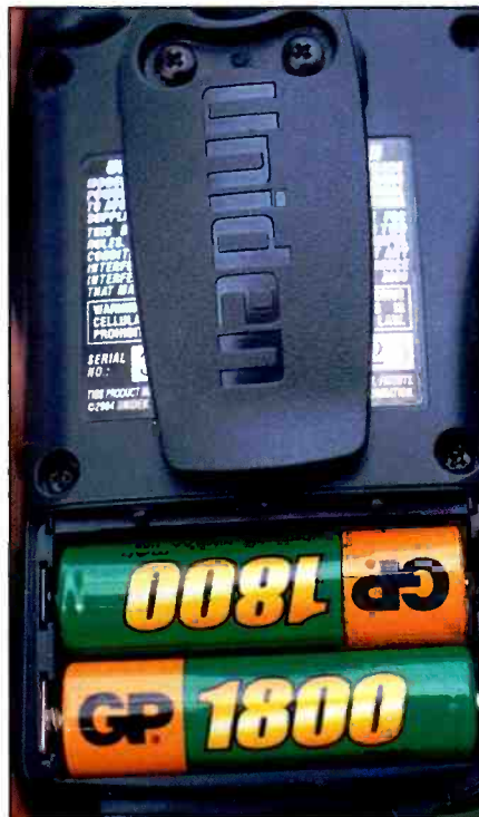
The supplied NiMH batteries lasted for six hours of continuous scanning.
