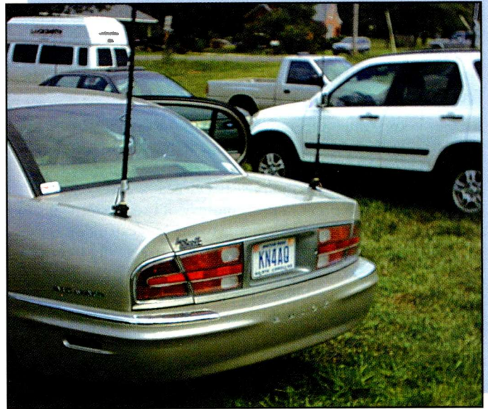
Gary Pearce, KN4AQ, editor of the SERA Journal , uses an outbacker HF antenna attached to the rear section of his vehicle by an L-bracket. This type of antenna utilizes taps that allow the user to easily select various frequency ranges from VHF to HF. Gary told me that his current antenna set-up works great and he gets good signal reports.
