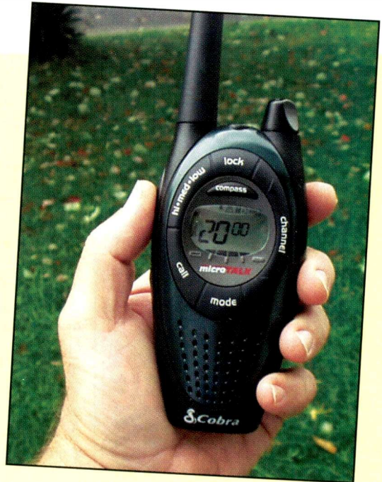
The Cobra PR4250 WX handheld FRS/GMRS transceiver is a full-featured radio that will keep you in touch around town or on the trail. You do need a license to operate on the GMRS.
