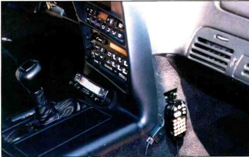
This remote head location is just too low for you to drive and change channels safely.
