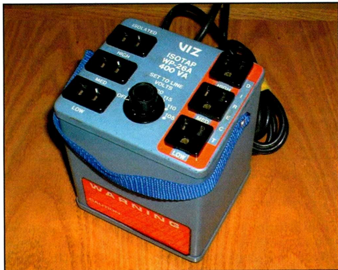
Photo C. This VIZ model WP-26A Isotap is a basic isolation transformer featuring multiple sockets for both isolated and non-isolated direct AC power connections. Various taps on the transformer offer three voltage choices for each side: high, medium, and low. A switch permits further "fine tuning" for higher or lower voltage settings. The unit was purchased from a closing TV shop for $20.
