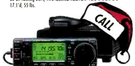
IC-706MKIIG The 160-10M + 6M, 2M, 70cm Mark II G is constructed for stable, quality output with low IMD and spurious emissions. Tone squelch, DSP, auto repeater and 107 memories. 6.56" w x 2.28" h x 7.88" d, 5 lbs, 6 oz. FREE RMK706* with purchase.
