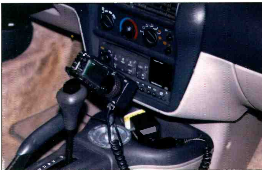
A convenient, yet still low, remote-head installation.
