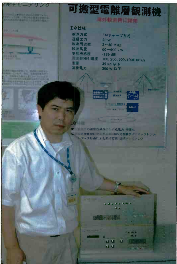
Dr. Takashi Maruyama with the FM Chirp portable XMITR/RCVR package for ionospheric research in the field.
