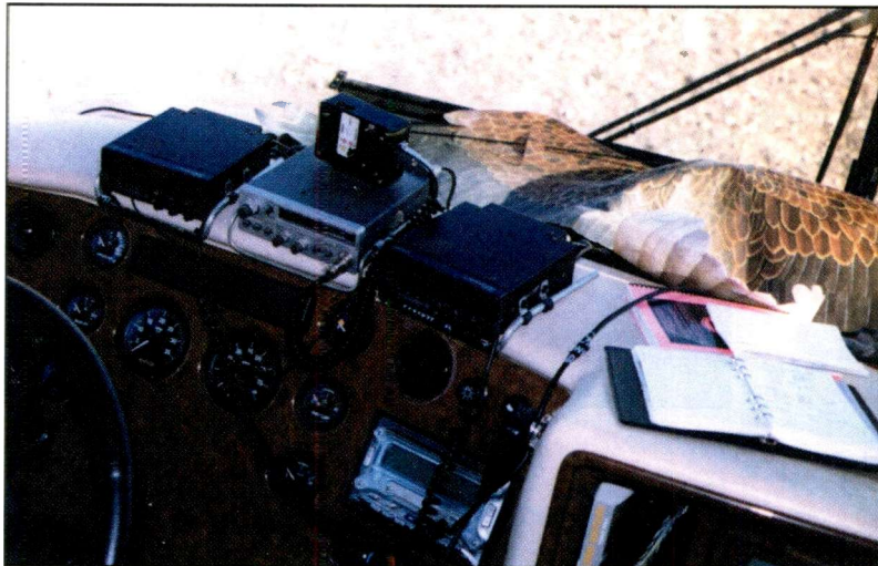
Here's a good "up high" motorhome radio installation, but remember to always be careful not to get the mic cable tangled in the steering wheel when you drive!
