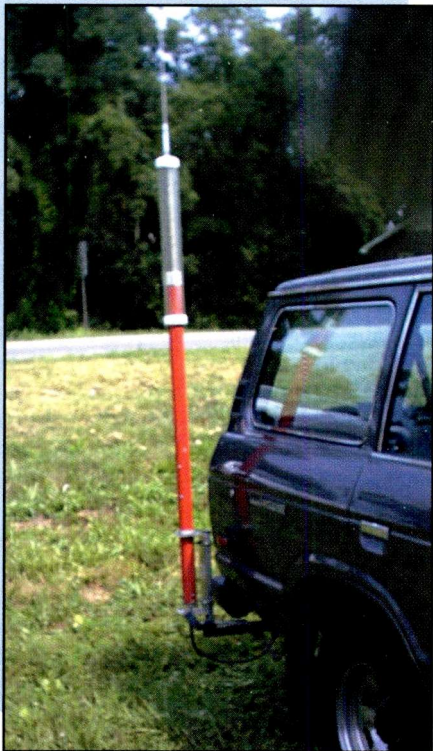
This type of mobile antenna requires a sturdy mount. The mount can be secured to either the frame of the vehicle or a receiver hitch-type bracket. Either will provide a strong support for the high wind load that this antenna will surely encounter.
