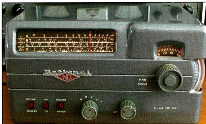
Photo A. National’s SW-54 shortwave communications receiver is a good example of an AC/DC set that requires extra attention before it can be used safely! (Photo courtesy Ed Engelken)
