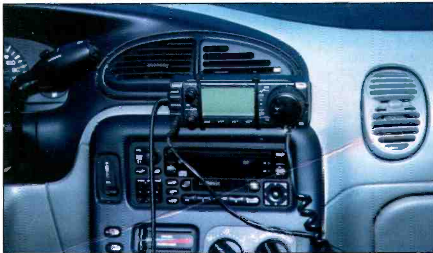
Here's N9ZGE's mobile installation with the remote head safely mounted high on the dash.
