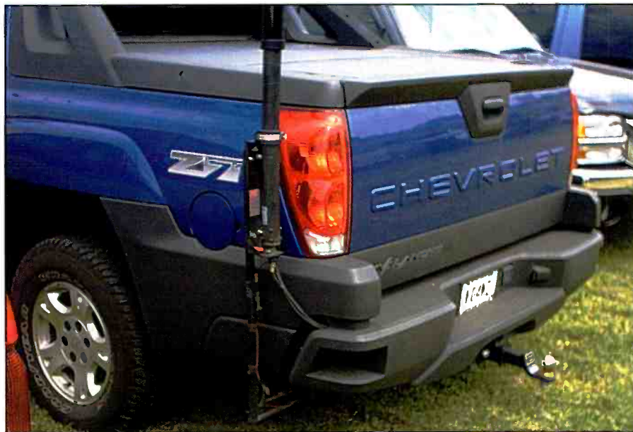
Notice how the power wires have been secured to the mounting bracket, preventing any movement of the wires that could cause a break in the connection. The coax cable is routed in an area free of moving parts.
