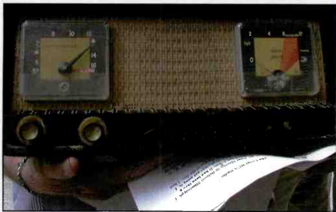
Photo 3. This rare Seferics radio made in Texas could detect approaching severe thunderstorms.
