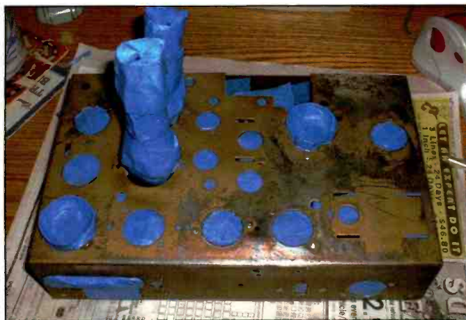
Photo G. Areas not to be painted must either be removed or taped over.
