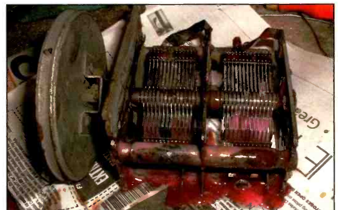
Photo I. The tuning capacitor was also given a good cleaning with Naval Jelly to remove most of the rust and to clean the aluminum plates.
