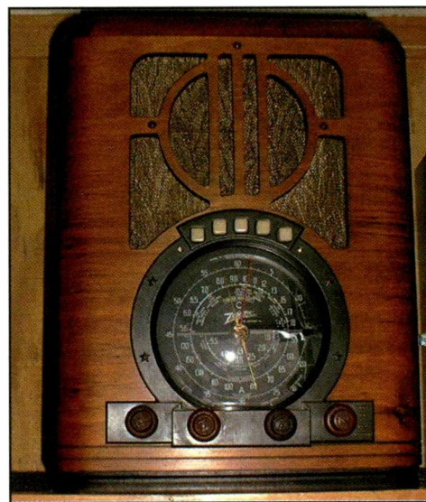
Photo B. This 1939 Zenith 6S330 tombstone sports the “Stars and Bars” escutcheon with Zenith’s “Tip-Touch Tuning” pushbutton preset station selectors.
