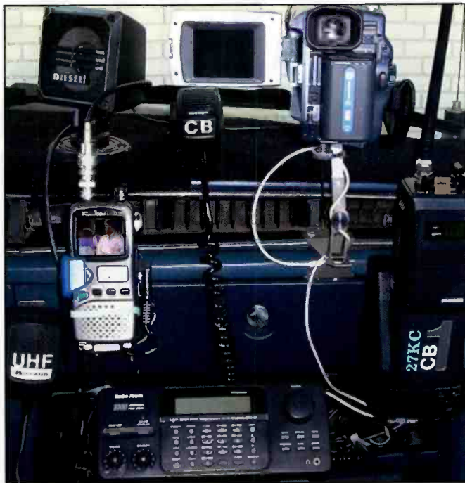
Receivers and video setup inside the author's storm intercept vehicle showing the wide range of equipment needed to do the job safely. Radios, from right to left, are the ICOM R-3 receiver with built-in video/television, RadioShack PRO-2035 scanner, and Maxon 27 KC CB walkie-talkie. Also shown is a Sony digital camera and Diesel extension speaker.
