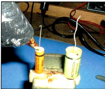
Photo O. Heated hot glue is injected into the capacitors to seal them and replicate the original wax fillers.
