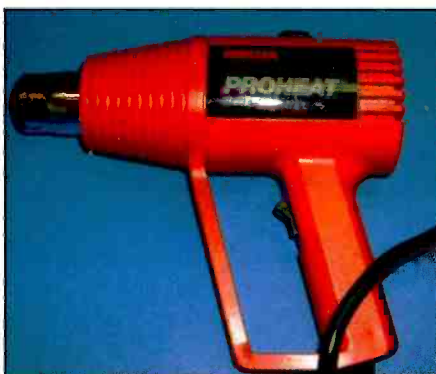
Photo H. Rebuilding old wax caps requires a means to heat and soften the old wax.
