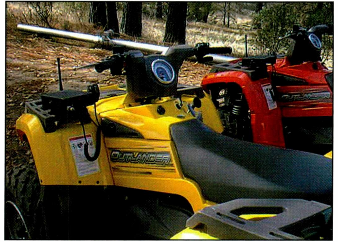
Here's a closer look at the perfectly functional RadioShack 19-1210 MURS transceiver installations. Notice the back-of-set rubber duckie antennas.
