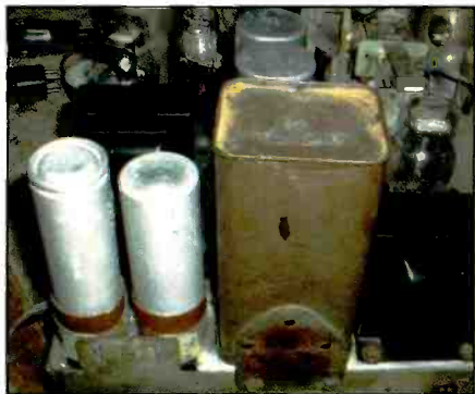
Photo E. The large filter and metal capacitor shells on the Philco 16B.
