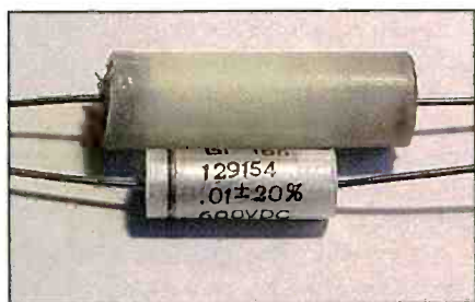
Photo R. Examples of Mylar caps resized using Glowstick tubing. (Photo by Bill Meachum)
