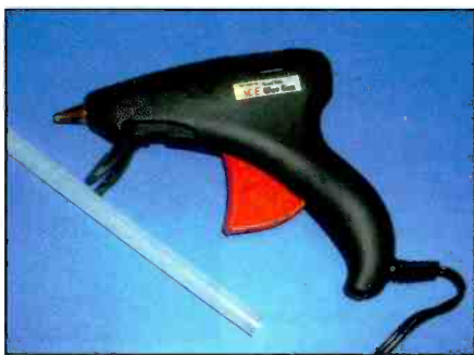
Photo I. Instead of wax, the caps are resealed using hot glue sticks.
