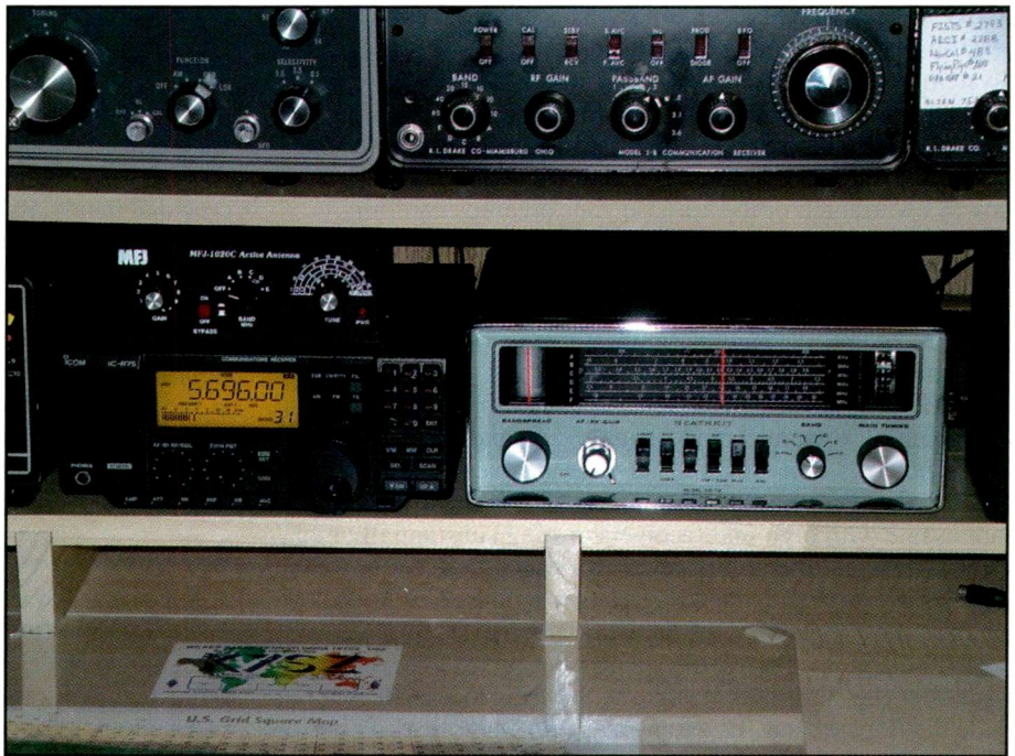
A brand new Heathkit GR-78 SW receiver I just built from a kit about a month ago sits next to the ICOM R-75
