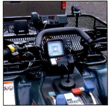
This is another of Paul's quads (sitting on the trailer) with a 19-1210 installation just above the handlebar, on the front basket.
