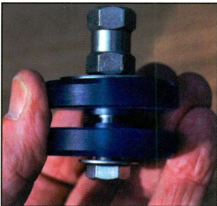
Here's a much more secure 3/8-inch x 24 mount where the bolt goes all the way through.
