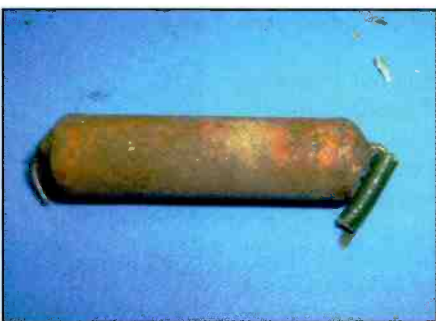
Photo J. Tube sets run warm, and dirt and dust will readily stick to the wax capacitors, making them hard to read.
