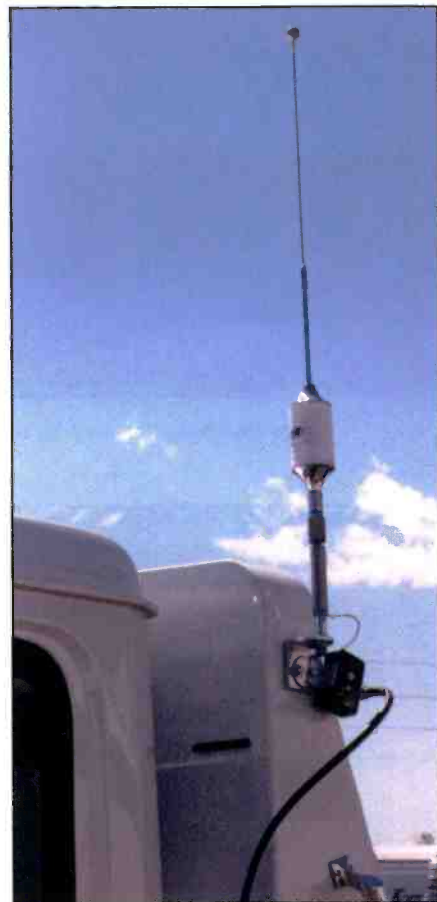
Here's a Hustler brand center-loaded whip with matching network at the base.
