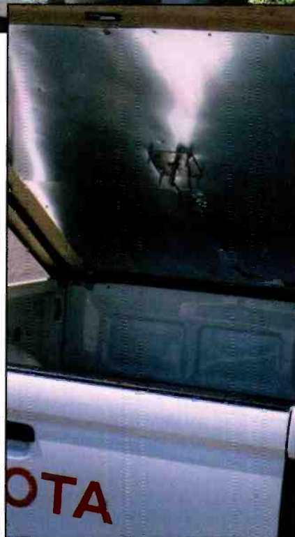
Here's N6VNI's way of mounting the ATAS-100 in the center of a metal lined fiberglass bed cover. He gets great results from 40 to 10 meters!
