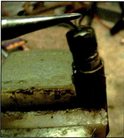
Photo M. Needle-nose pliers are used to pull the ends free of the heated capacitor body. An unsharpened pencil is used to push the old capacitor body out of the shell.
