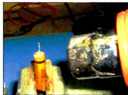
Photo L. The hot air gun is used to lay heated air around the capacitor body. Once sufficiently heated, the wax softens, permitting the capacitor can be easily gutted.
