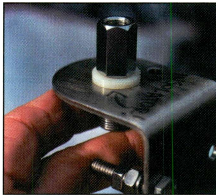
Watch out! This fitting will fail under the load of a heavy coil antenna.
