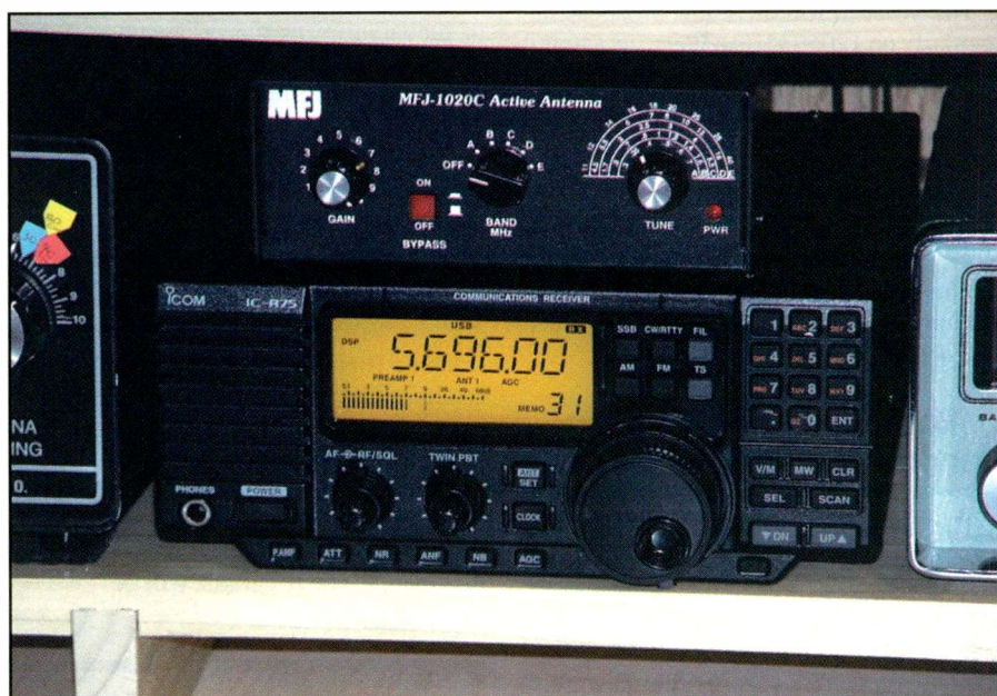
Here's the R-75 at my operating position. I am using the MFJ-1020C Active Antenna as a preselector, NOT an active antenna.
