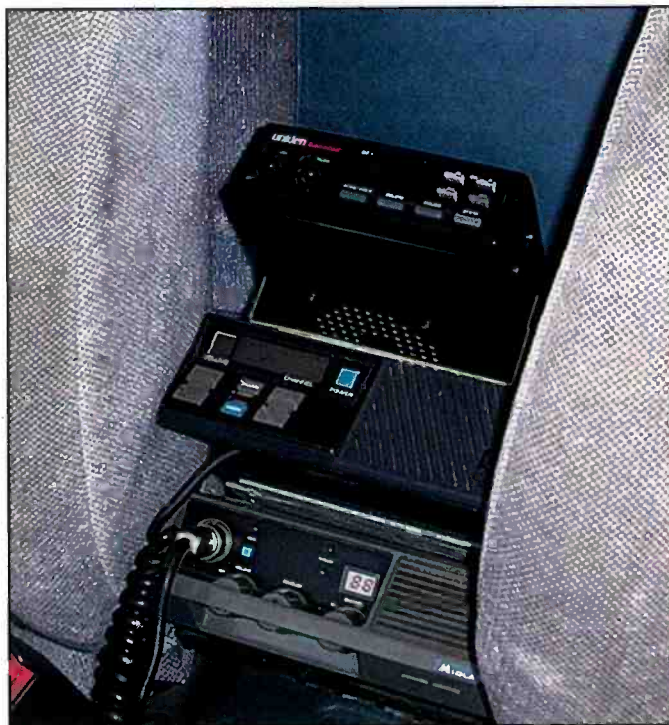
Two-way radio equipment is mounted between the seats, including a General Electric 30-watt VHF transceiver and a UHF GMRS unit. Also shown is a Uniden BC-1 pre-programmed service search scanner.
