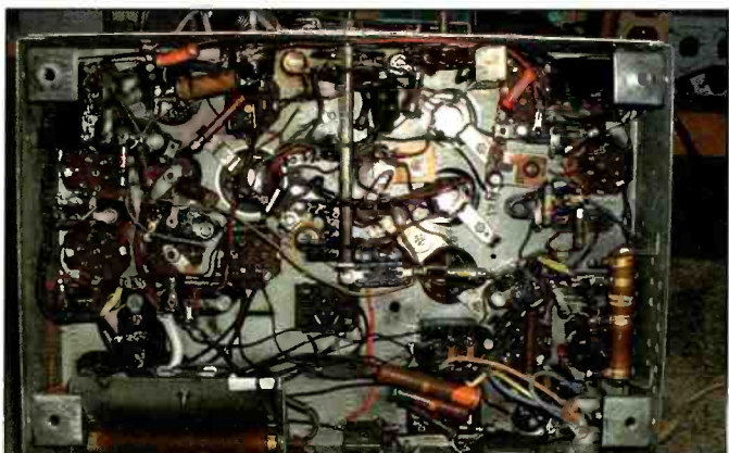
Photo D. This 16B chassis was also restored using techniques that maintained the original factory appearances.
