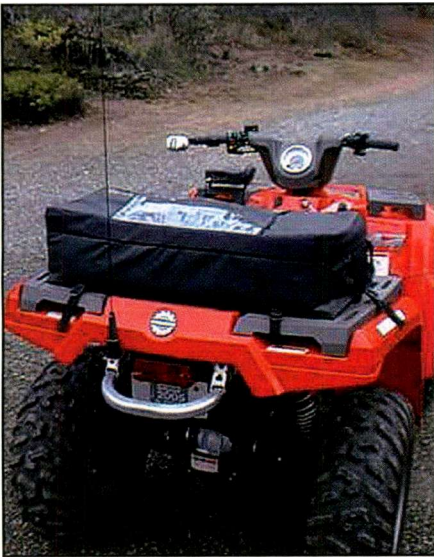
Notice Paul's upgraded MURS/2-meter VHF antenna installation on the rear bar.
