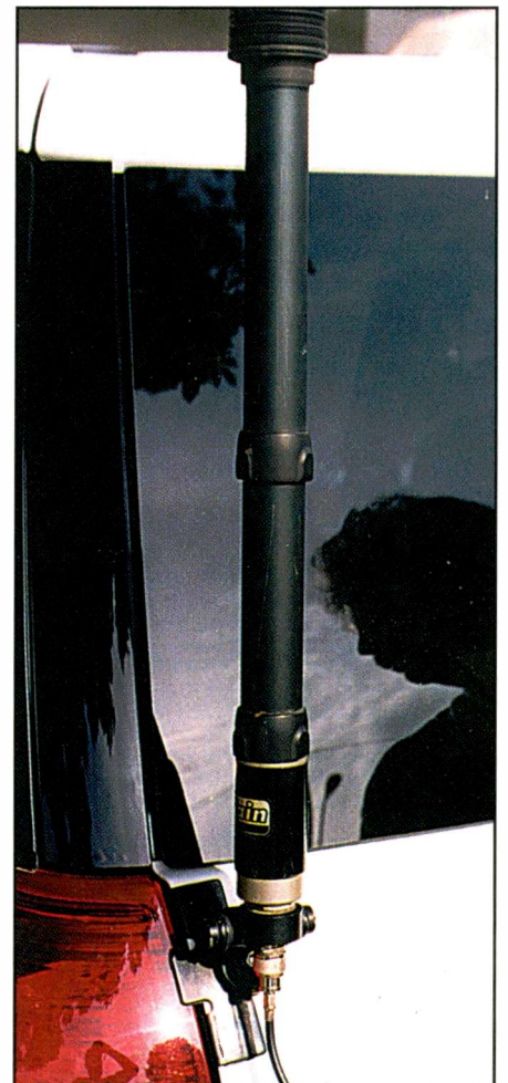
A strong lip mount on your vehicle will hold a variety of HF antennas.
