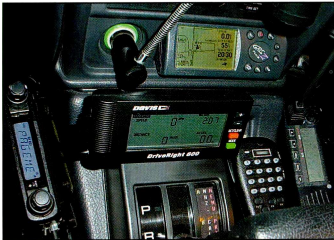
This is one beautiful installation of the DriveRight 600 display console! We installed it in our project vehicle's center console, fitted among the various other telematics devices on board, just below our GPS mapping display. Having the two data displays together makes for easier viewing of both, at a glance.
