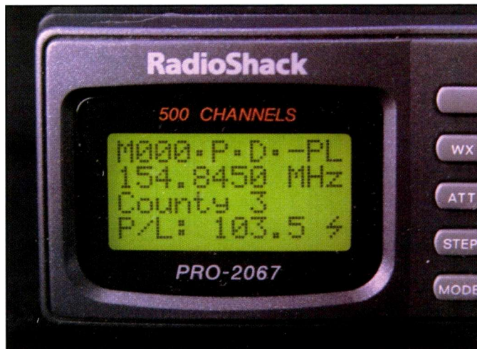
Some of the newer receivers with built in CTCSS can display the tone right on the main display. This can be very useful for identification of the transmitting station.
