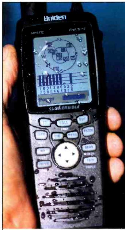
This handheld Uniden VHF marine radio is also a GPS unit!
