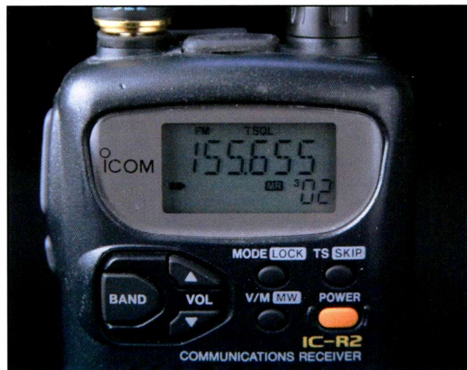
Other receivers just let you know that the tone squelch is engaged. Check the top center of this IC-R2 display.
