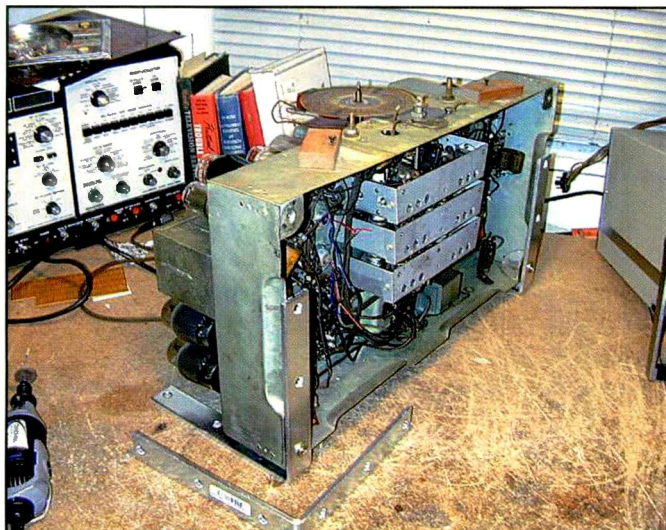
Photo A. Some things are so obvious you have to wonder why you didn't think of them! So it is with Phil Nelson's simple and quick way to support a large chassis on the bench. The chassis undergoing restoration is a large Midwest console, a very desirable deco-looking set. (Photo courtesy www.antiqueradio.org )
