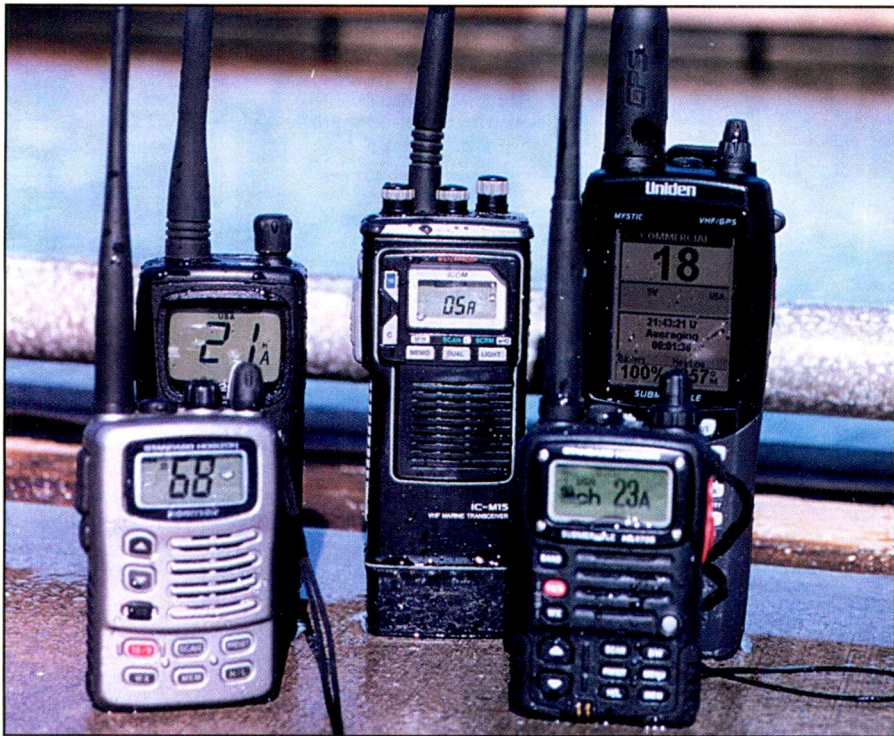
All five handheld marine VHF radios survived an hour in the water with no leaks.
