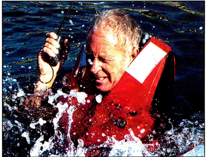
Each radio was turned on and held under water for two minutes.
