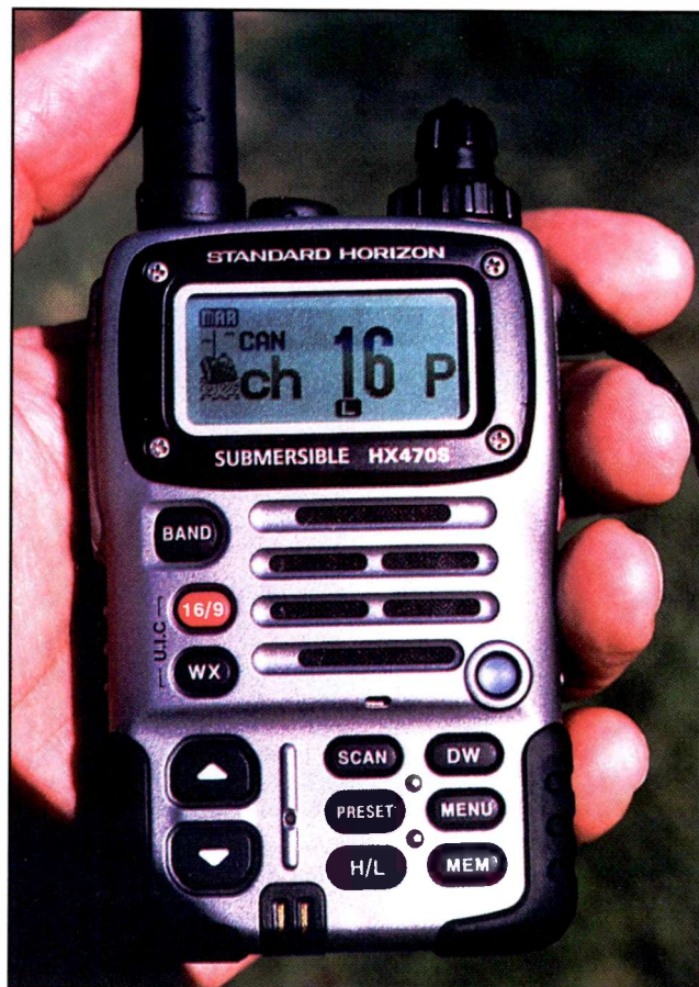
The new, but not FCC-approved, marine VHF handheld from Standard Horizon with DSC capabilities.
