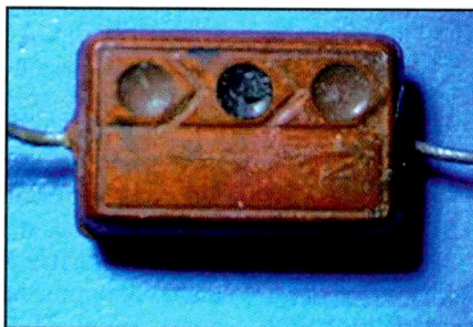
Photo A. This early mica capacitor uses a simple, but obsolete, RMA 3-dot marking system. With the indicating arrow(s) pointing right, the color-coded dots are read left-to-right as brown-black-brown. According to Table 1 , this is a 100-mmfd (100pF) capacitor.
