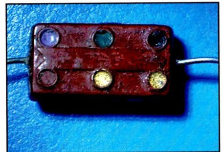
Photo C. This six-dot mica capacitor uses the obsolete RMA 6-dot marking standard. With the capacitor placed so that the arrows point to the right, the first three dots read violet-green-black going in a clockwise direction.
