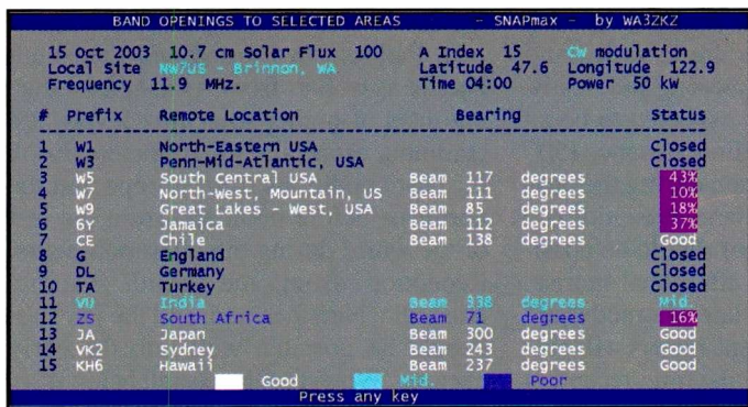
Figure 4. Band openings from various locations around the globe, on 11-MHz shortwave at 0400 GMT. The Pacific Region is wide open into the Pacific Northwest of the United States.
