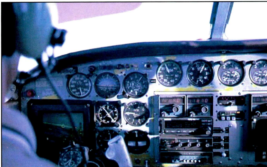
A view of the cockpit of the Beech QueenAir used in the initial testing of WAAS in Alaska. The left side of the panel shows a WAAS display unit.
