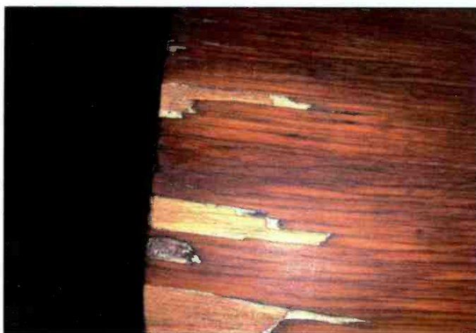
Photo D. Three areas missing veneer are patched using roughly cut in and glued veneer patches. Gaps were later filled with wood filler and then sanded after the filler dried.
