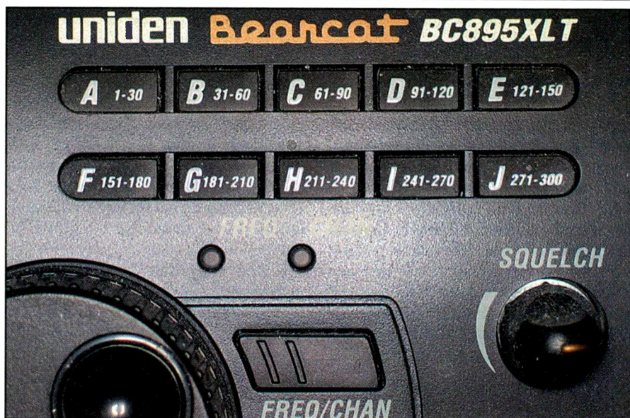
This receiver from Uniden features a separate set of 10 keys for convenience. Some Uniden receivers have used these extra keys to get a total of 20 banks, which is very convenient for splitting up your channels and grouping them into logical blocks.
