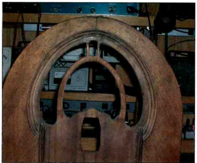
Photo K. Here's the finish layer of veneer in place and stained to match. It's starting to look as good as new at this point, thanks to some final sanding and trimming.
