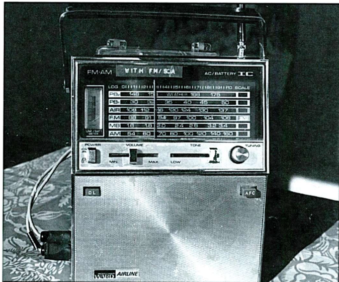
Front view of a vintage Wards Airline radio showing SCS "in" and "out" plugs using the radio's "MPX" out jack (a jack not found on modern radios) and its audio-in jack.
