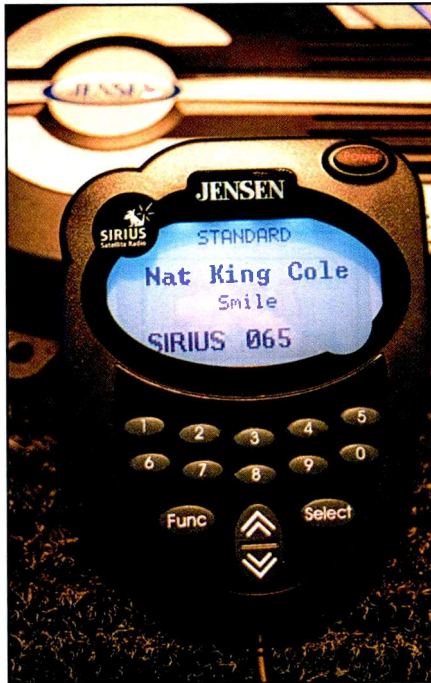
The backlit LCD controller at night. It has four levels of dimming.
