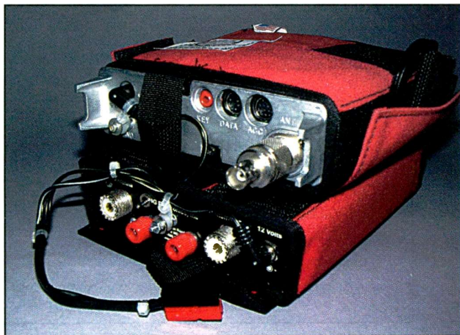
This is a shot of the rear end of my portable/mobile HF SSB/CW/DATA station, a Yaesu FT-817/LDG Z-11 autotuner. Both are DC powered and have permanently attached power cords that are terminated in Anderson PowerPoles for attachment to a West Mountain RIGrunner.
