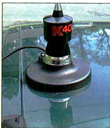
The completed K40 and Magnamount ready to hit the road. I like to call this a K40 antenna "system" because it's so versatile: mag-mount, trunk-lip mount, or if you're brave, drill-a-hole-through-the-roof mount!
