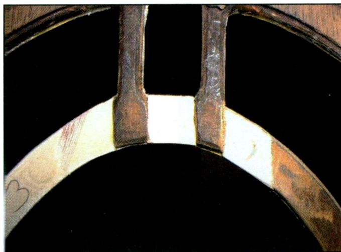
Photo H. The micro-plywood is carefully cut, following the tracing outline. Fine tuning will be done using sandpaper.
