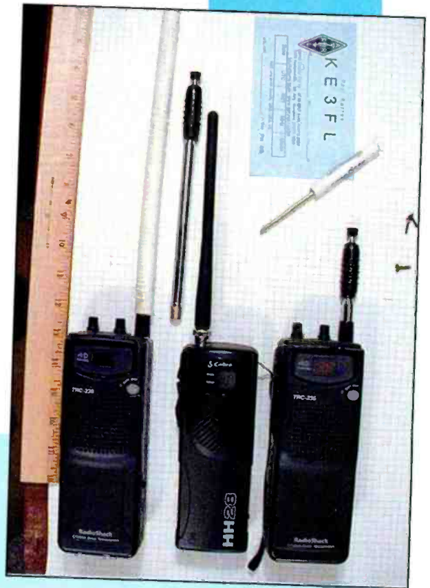
CB with semi-flex antenna, CB with rubber ducky, and normal CB antenna collapsed.
