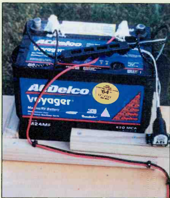
The AC Delco battery and Casco 12 Vdc outlet.
