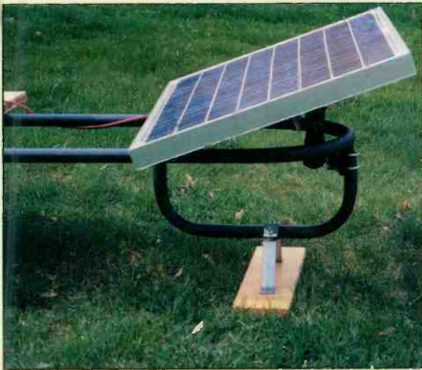
Detail photo of the Kyocera panel and foot keeping the dolly off damp ground.
