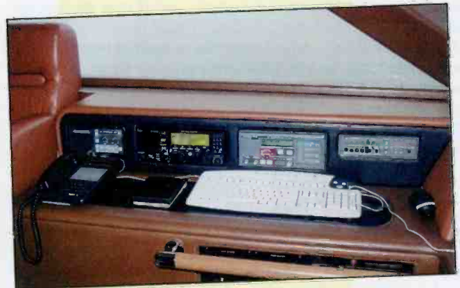
A modern shipboard DSC station for both HF and VHF DSC calls.
