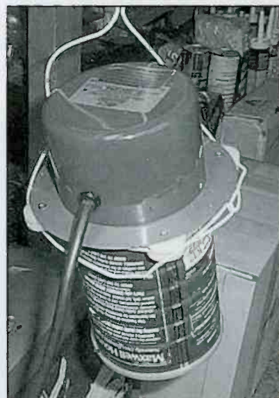
Rich Shiver's homemade parts cleaner, using a Magic Fingers motel-bed massager mechanism and coffee can filled with sand.
