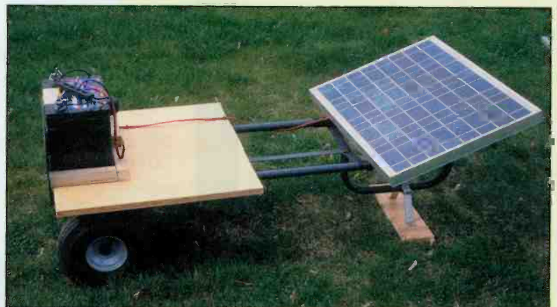
Our completed project with the Kyocera KC35 panel and AC Delco Voyager battery.
