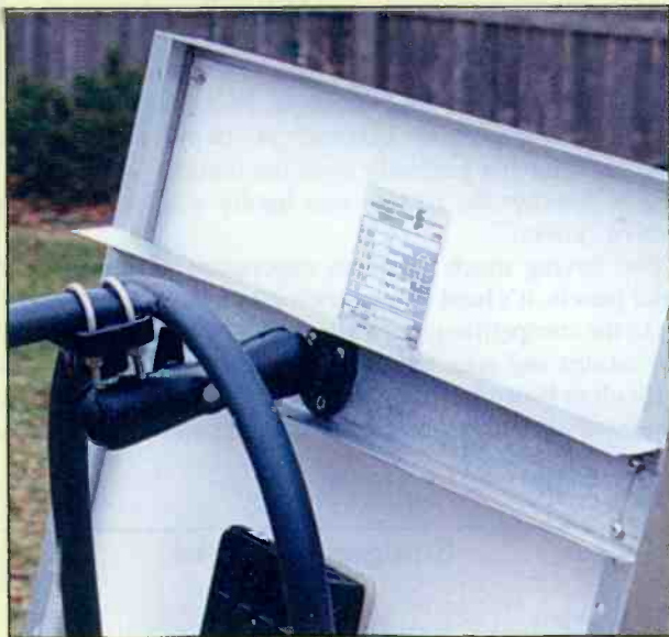
The RAM-111 universal mount attached to the metal strip offers superb versatility.
