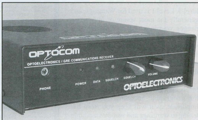
The front-mounted volume and squelch controls can be over-ridden by software controls. You have to keep this in mind when you start wondering why the radio is making noise with the volume turned all the way down!
