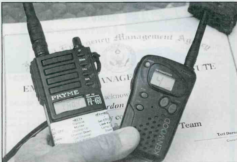
GMRS (left) and FRS may indeed intercommunicate on FRS channels 1-7.
