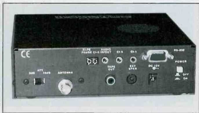
The connections on an Optocom receiver are quite extensive. This is one of the only computer-controlled receivers or "black box"-type radios that can at least function without the computer connected.
