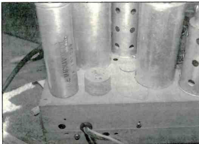
Photo 7. Wood plug is mounted over the original mounting hole using wood screws through the bottom. They are pan head screws positioned so their heads grip the metal edges of the mounting hole.
