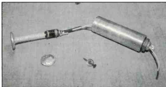
Photo 11. A wood dowel running the inside length of the capacitor is the secret of how it is put back together using sheet-rock screws.
