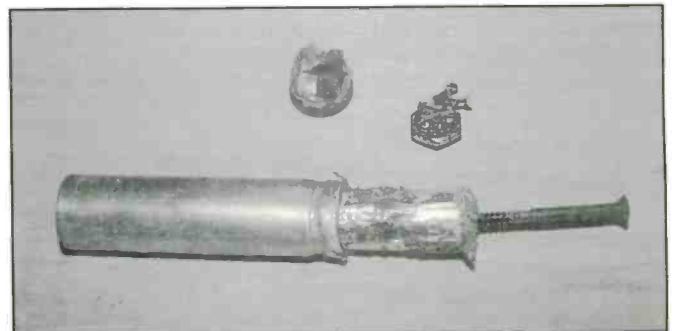
Photo 4. A large wood screw driven into the capacitor body allows the innards to be pulled free of the shell and discarded.
