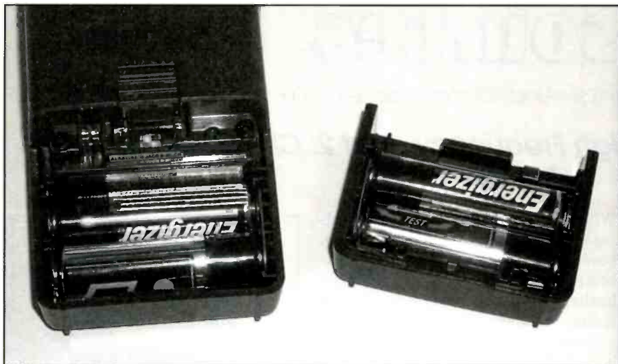
At last — standard AA batteries in a trunktracker scanner! The unusual “clamshell” holder splits off the back and holds two of the four batteries.
