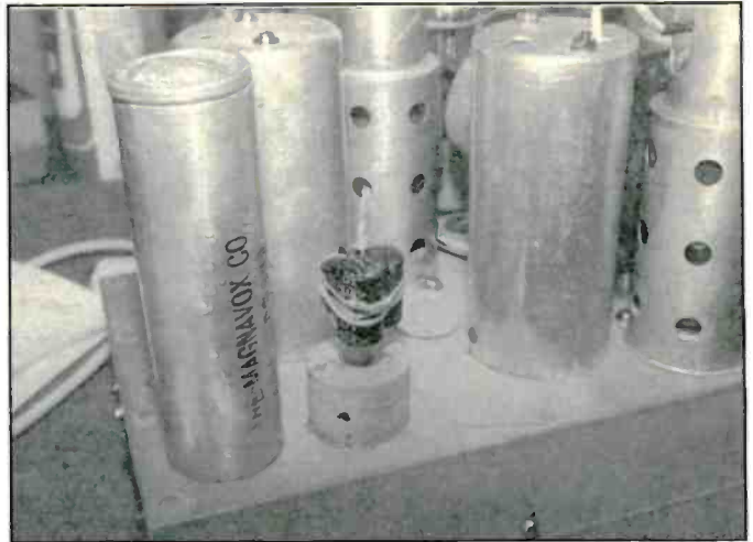
Photo 8. Replacement electrolytic capacitors are in place. The leads run through the hole produced by the pilot drill bit in the hole saw. Everything is carefully taped and insulated before the shell is replaced and screwed to the mounting plug.
