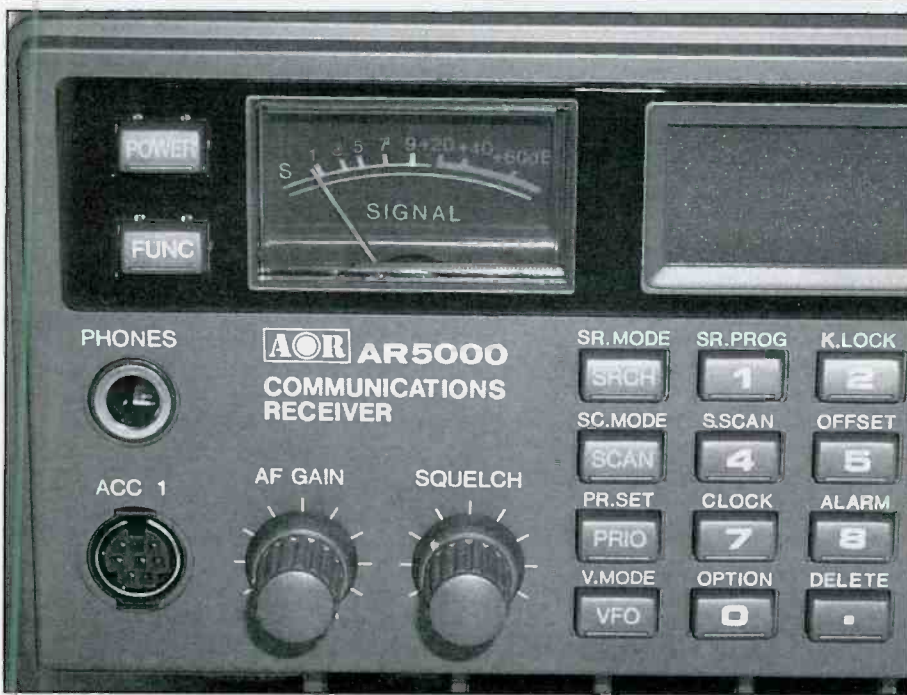
The unique front-mounted accessory jack provides a lot of options including a discriminator output if you need one.
