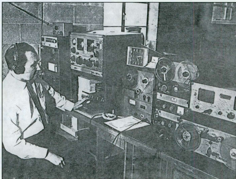
WBTV engineer Lon Chaney monitors Radio Moscow in the basement of his home in Union County. Lon has three receivers and three tape recorders. Depending on reception, he could have as many as three recordings at once. Later, he rigged a device which automatically recorded from the receiver giving the best reception.
