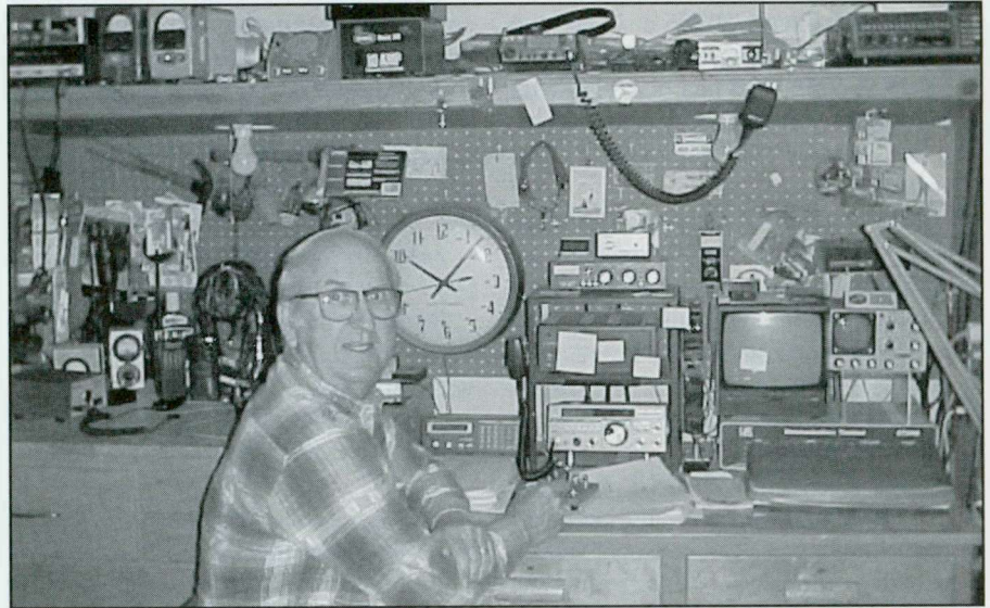
Longtime reader Bill Farley (New Mexico) sent a picture of his shack which includes several scanners (RadioShack, Uniden, etc.) and an ICOM VHF/UHF transceiver, and a Yaesu 757GX transceiver attached to a HAL CT-2100 CW, RTTY terminal.
