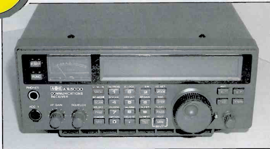
The AR5000 Plus 3 provides a lot of radio in a small space. The speaker is bottom-mounted, but directed forward through the grille at the bottom. The elevated front feet can be removed if desired so the radio sits level on the table.
