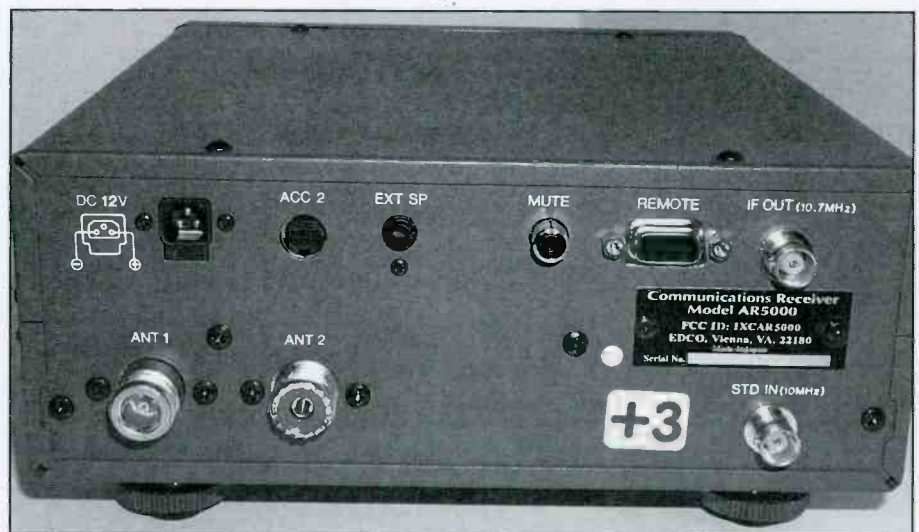
The rear panel of the AR-5000 Plus 3 is quite well-equipped. Note the "+3" sticker which is the only outward indication that this receiver is equipped with the additional features. Also note the two antenna jacks — a type N and an SO-239.
