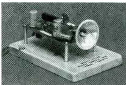
The author's prototype of the SentryStrobe was mounted on stand-offs to block off wood for testing. The dark object between the two capacitors is the 500-ohm, 25-watt ceramic power resistor (R6) used in the power-supply circuit.
