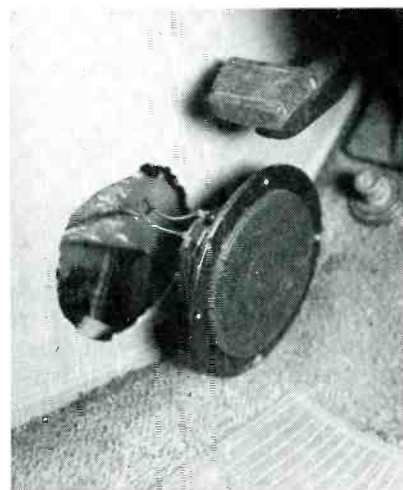
FIG. 12—CONFIRM THE CLEARANCE space when mounting speakers in door panels or front kick panels by removing the panel and making a measurement.
