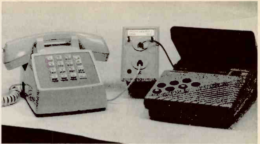
FIG. 5—SETUP FOR TESTING AN ANSWERING MACHINE with phone helper.
