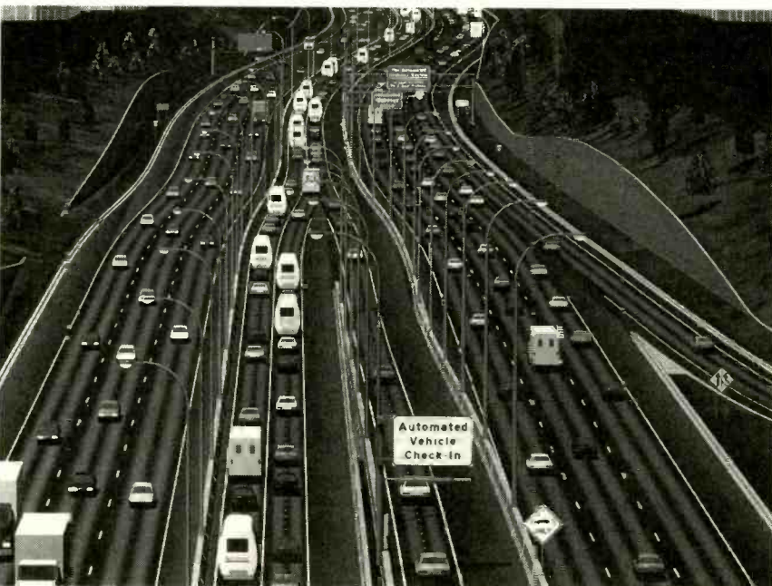
AHS would use dedicated HOV lanes separated from regular traffic lanes. Note the closer vehicle spacing allowed by AHS.
