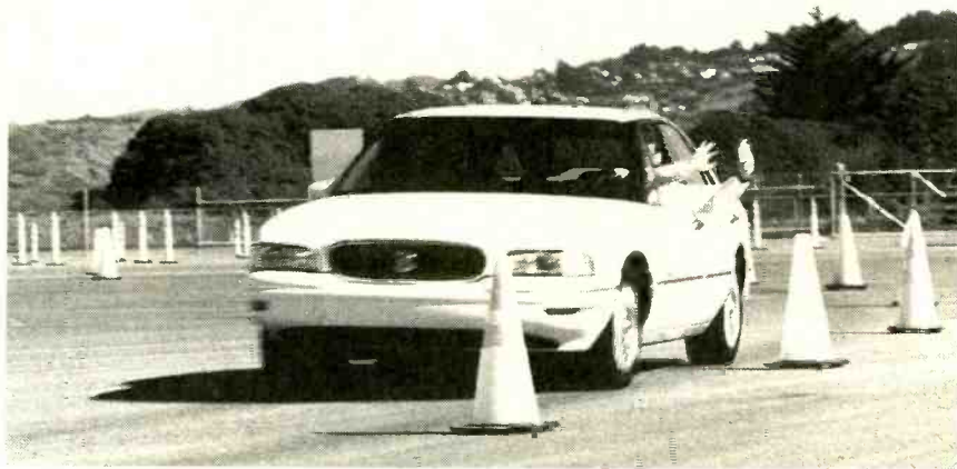
AHS technology used on the Buicks allowed them to be driven "hands-off" and "feet-off."
