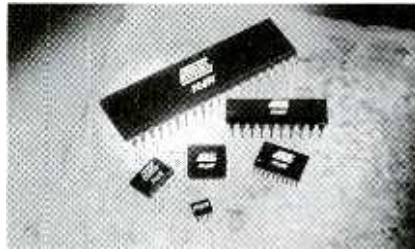
AVR chips have built-in timer-counters that can be used to keep track of how long something takes or to count the number of occurrences of some event.
