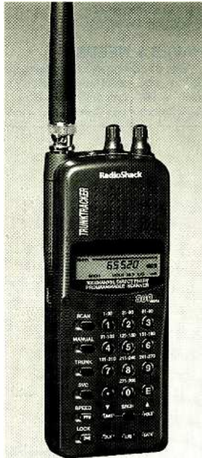
The PRO-90 Trunk Tracker from RadioShack is a 300-channel triple-conversion handheld unit.
