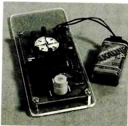
The author's unit was simply mounted on spacers to a small section of Plexiglas. Note: When using the unit, it is important to keep the sensor horizontal.
