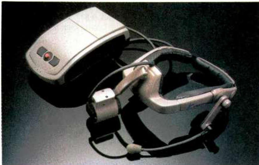
The Mobile Assistant II is a voice-activated Pentium system that you wear.
