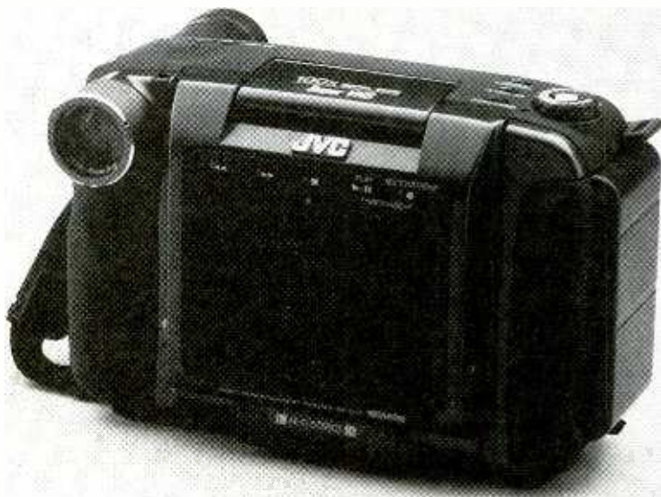
JVC's new GR-SV7 S-VHS camcorder features both a color LCD screen and a conventional viewfinder
