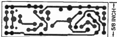
Fig. 2. If you'd like to etch your own board for the Transmitter, use this template.
