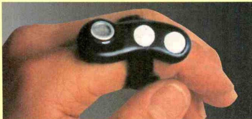
The Ring Mouse is designed to be worn comfortably on the index finger. Its two buttons are within easy reach of the thumb. Note the ultrasonic transducer on the right of the unit.
