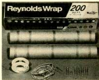
Here are all of the items need to assemble your own Cardboard Tube Radio.
