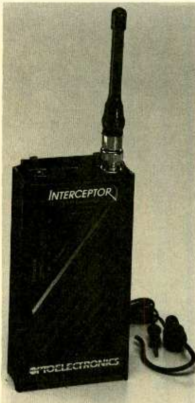
The Optoelectronics R10 FM Communications Interceptor lets you search for signals from any FM transmitter over 30 MHz to 2 GHz. Tuning is automatic; the R10 locks on instantly to the nearest transmitter.
