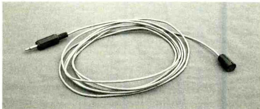
The electret microphone element that's used to pick up audio from the piano is mounted to one end of a length of microphone cable and a phone jack is connected to the other end.
