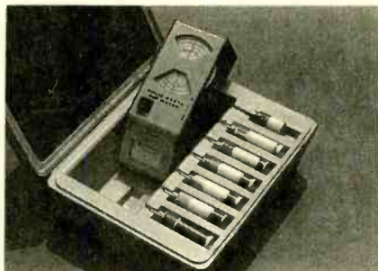
This Heath dip meter comes with a variety of coils so that it can cover a wide frequency range. Although you have to build it yourself, if done properly it is a quality instrument.
