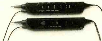
A logic probe (top) and a logic pulser (bottom) are the most useful pieces of equipment to have around when troubleshooting low-speed logic circuits. The probe shown here can test both main families of logic and comes with switch-selectable pulse stretching. The pulser shown here can send out single or multiple pulses.
