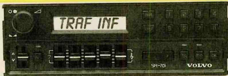
An RDS receiver can find the exact information you wish to listen to and indicate the program content in alphanumeric form on its display.
