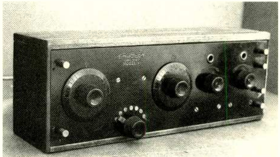
The front panel of Ray Shetrone's Crosley VI . Note the tube-viewing "portholes" just above the two-filament rheostats at right.
