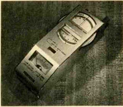
This is an older model impedance bridge. It can be used by SWL's as well as ham operators because it contains an amplifier to boost the signal from any low power oscillator for test purposes.
