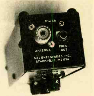
Looking down at the MFJ-204B you will see a FREQUENCY output jack as well as an ANTENNA output jack. It allows you to read the operating frequency on an accurate meter for fine tuning the antenna.
