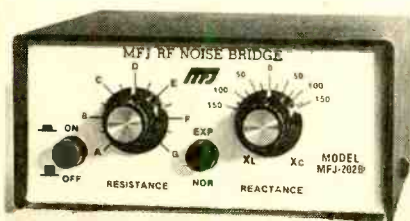
This MFJ RF noise bridge comes with its own individual calibration chart for the most accurate measurement of antenna resistance possible.
