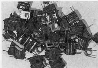
Surplus inductors are often color-coded like resistors, starting at the top. Yellow-purple-brown means 470 \mu H.
