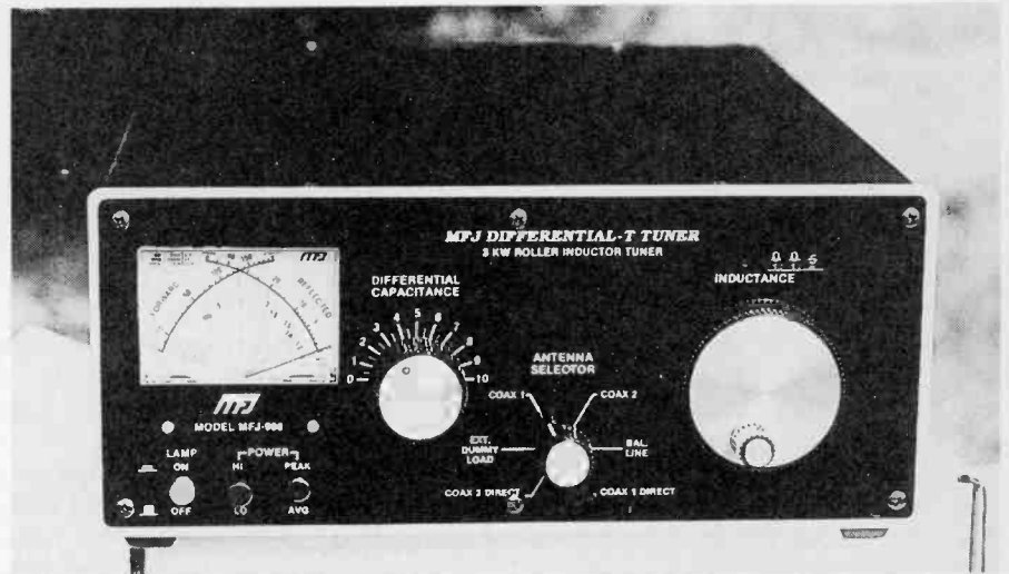
The MFJ-986 antenna tuner covers the entire region from 1.8 MHz to 30 MHz, including the WARC bands. Because of its roller-inductor design, it can accommodate a wide range of impedance values continuously over its entire operating range.
