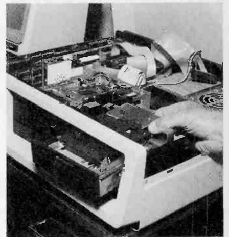
If there is a drive installed above the existing hard-disk drive, remove it first. Do not try to slip the hard disk out from under another drive.
