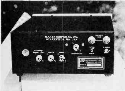
All input and output connections for the MFJ-986 are found on the rear panel; included is a pair of ceramic insulators for balanced antenna transmission lines.
