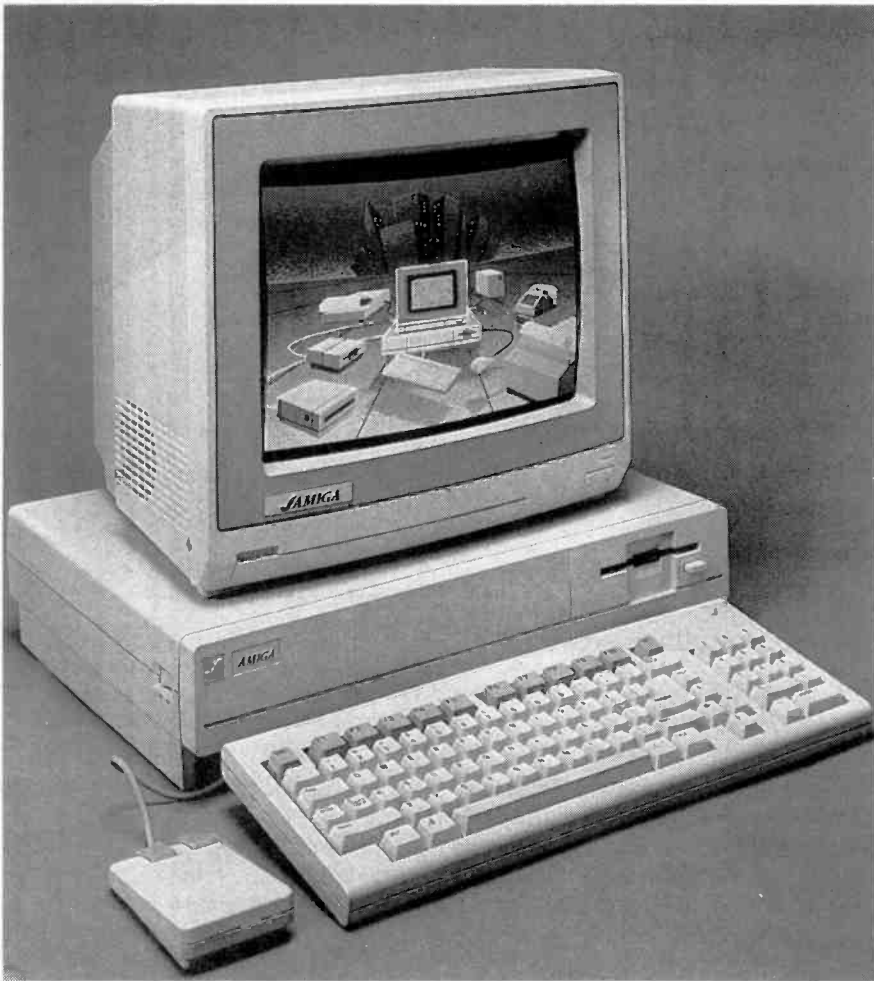
A game-player's dream come true, the Amiga's features include arcade-quality 4,096-color graphics, two mouse/joystick ports, four-voice digital stereo sound, multitasking capability (you could conceivably play two games at once), and even left- and right-audio outputs for driving a stereo-sound system.
