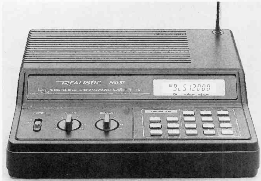
Radio Shack's Realistic PRO-57 is a small, ten-channel programmable scanner that provides frequency coverage from 30 to 54 MHz, 138 to 174 MHz, and 380 to 512 MHz, with 1.0- \mu V sensitivity in all bands; it lists for $139.95.
