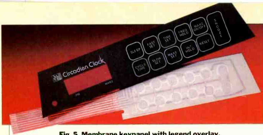
Fig. 5. Membrane keypad with legend overlay.
